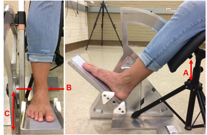
Figure 3. Experimental setup. The examiner adjusts the leg rest (A), heel rest (not depicted here), and footrest, to align the ankle with the system CoR (B + C) before starting the testing procedure.
