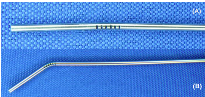
FIGURE 1: (A) UNBENT TENDON-DRIVEN ACTIVE NEEDLE USED IN THIS WORK TO DETERMINE TISSUE MOVEMENT DURING NEEDLE ACTUATION. (B) BENT CONFIGURATION OF THE ACTIVE NEEDLE OBSERVED IN AIR.
