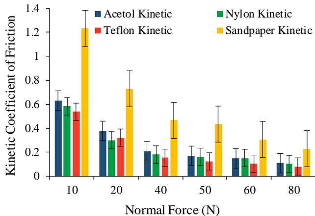
**FIGURE 5:** KINETIC COEFFICIENT OF FRICTION OF ACETOL, TEFLON, NYLON, AND SANDPAPER OVER SIX DIFFERENT NORMAL FORCES
