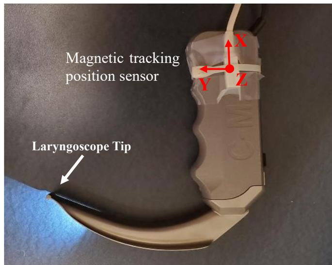
**FIGURE 1:** C-MAC LARYNGOSCOPE WITH MAGNETIC TRACKER ATTACHED ON THE UPPER LEFT SIDE OF THE HANDLE
