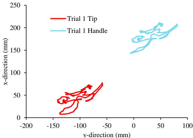
**FIGURE 4: LARYNGOSCOPE HANDLE AND TIP MOTION PLOT FOR TRIAL ONE**
