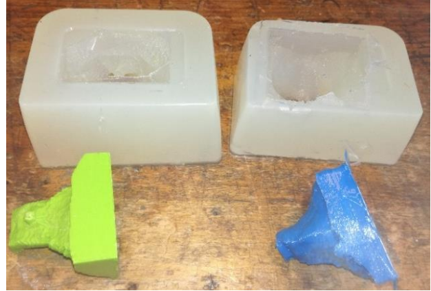
FIGURE 3: TWO SILICONE RUBBER TRACHEOSTOMA MODELS AND THEIR CORRESPONDING 3D-PRINTED NEGATIVE TRACHEOSTOMA IMPRINTS.
