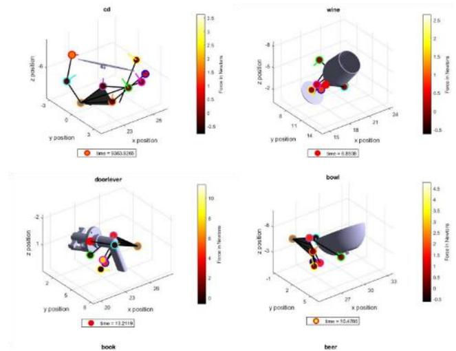
**FIGURE 5:** FRAMES OF GRAPHICAL REPRESENTATION OF GRASPING TASKS BY HUMAN SUBJECTS. A SKELETAL REPRESENTATION OF THE HAND ALLOWS EASY VISUALIZATION OF DIFFERENT HAND CONFIGURATIONS. THE COLOR INFILLS AT CRITICAL LOCATIONS OF THE HAND ILLUSTRATE THE CONTACT DYNAMICS OF THE HAND DURING TASK PERFORMANCE.
