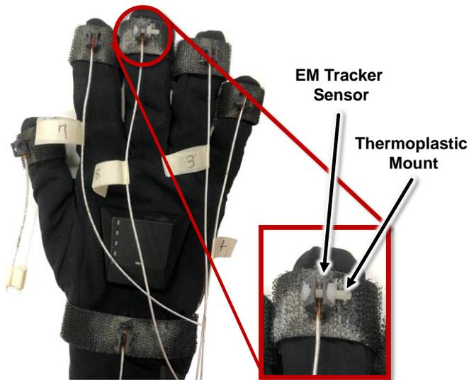
**FIGURE 2:** SENSORIZED GLOVE SYSTEM. ZOOMED-IN IMAGE OF THE MIDDLE FINGER SHOWS THE TRACKER SENSOR MOUNTED ON A THERMOPLASTIC ELASTOMER MOUNT, FASTENED WITH A NYLON SCREW TO PREVENT ELECTROMAGNETIC INTERFERENCE.
