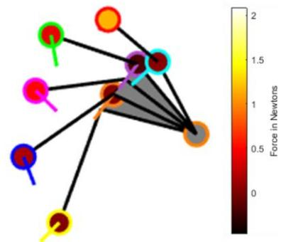
**FIGURE 4:** SKELETAL REPRESENTATION OF THE HAND WITH INFILLS REPRESENTING FORCE MAGNITUDES. THE COLORBAR ON THE RIGHT DISPLAYS FORCE VALUES AT DIFFERENT COLORS. OUTLINE COLORS OF THE CIRCLES REPRESENT CONTACT POINT LOCATIONS WITH THUMB, INDEX, MIDDLE, RING, LITTLE FINGERS BEING RED, GREEN, MAGENTA, BLUE, AND YELLOW RESPECTIVELY.
