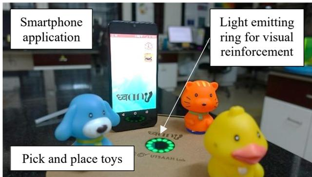
**FIGURE 2:** DEVELOPED CONCEPT OF THE RESPONSE SYSTEM
