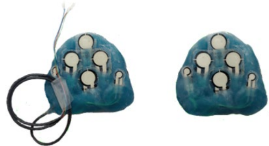
FIGURE 8: A TEMPORARY WIRE LEAD ALLOWED RE-PROGRAMMING OF THE MICROCONTROLLER. AFTER WHICH THE LEAD WAS CUT AND SEALED.
