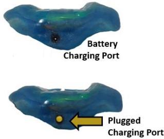
**FIGURE 6:** A RUBBER STOPPER SEALS THE CHARGING PORT.
