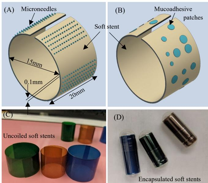
**FIGURE 1:** Self-uncoiling drug carrier platform- 'soft stent'. Schematic diagram of soft stent with conceptual drug loaded (A) microneedles, and (B) mucoadhesive patches; (C) cylindrical soft stent maintains its shape when no load is applied; (D) soft stent coiled and encapsulated in easily swallowable capsule shells.
