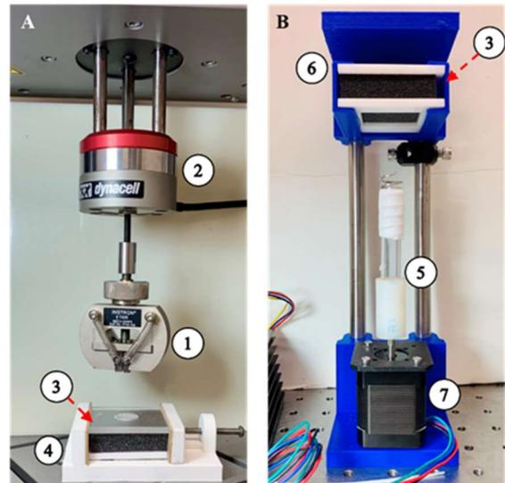
**FIGURE 2.** SETUP FOR SUTURE INSERTION A. STRAIGHT NEEDLE, B. HELICAL NEEDLE: (1) UPPER JAWS, (2) 2 KN LOAD CELL, (3) PHANTOM TISSIE AND TISSUE HOLDER (4) TISSUE MOUNT, (5) HELICAL NEEDLE AND COUPLER (6) VERTICAL STAGE (7) STEPPER MOTOR
