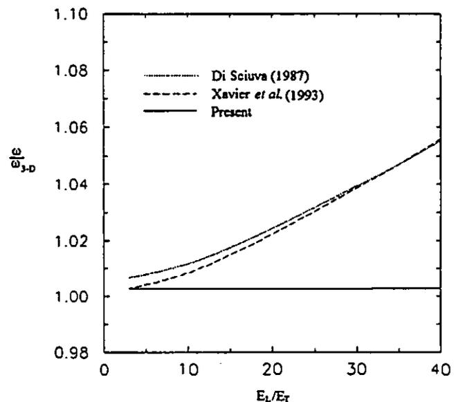
Fig. 6 Effect of lamina orthotropy on accuracy of natural frequencies for ( $0^\circ/90^\circ$ ) composite cylinders with  $L/R=1$ ,  $R/h=5$ , and  $m=1$ ,  $n=2$ .
