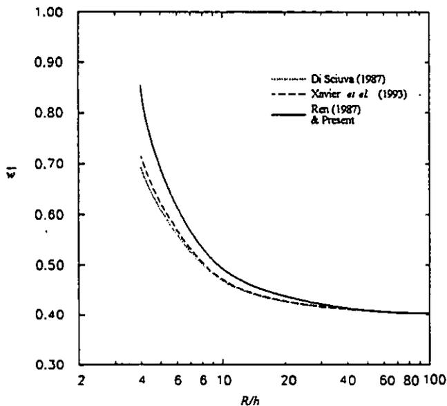
Fig. 5 Maximum deflection as a function of  $R/h$  in cylindrical bending of a ( $0^\circ/90^\circ$ ) cylindrical laminated shell under sinusoidal loading
