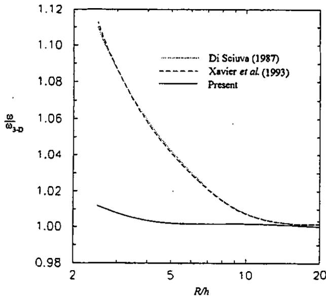
Fig. 7 Effect of radius-to-thickness ratio on accuracy of natural frequencies for  $(0^\circ/90^\circ)$  composite cylinders with  $L/R=1$ ,  $E_L/E_T=30$ , and  $m=1$ ,  $n=2$ .
