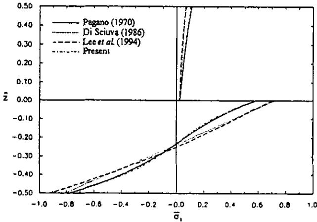
Fig. 3 Distribution of in-plane stress  $\bar{\sigma}_1(a/2, a/2, \bar{z})$  in a  $(0^\circ/90^\circ)$  square laminate with  $a/h = 4$  under sinusoidal loading
