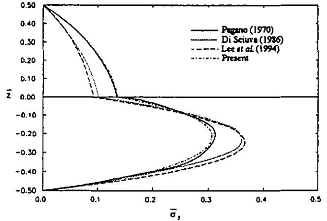
Fig. 4 Distribution of transverse shear stress  $\bar{\sigma}_5(a/2, a/2, \bar{z})$  in a  $(0^\circ/90^\circ)$  square laminate with  $a/h = 4$  under sinusoidal loading
