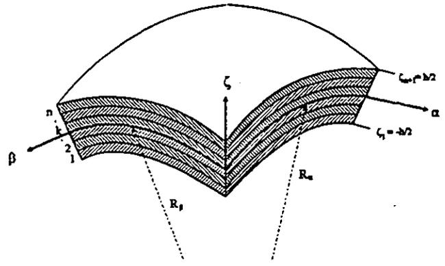
Fig. 2 Laminated shell geometry
