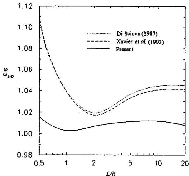
Fig. 8 Effect of length-to-thickness ratio on accuracy of natural frequencies for  $(0^\circ/90^\circ)$  composite cylinders with  $R/h=5$ ,  $E_L/E_T=30$ , and  $m=1$ ,  $n=2$ .
