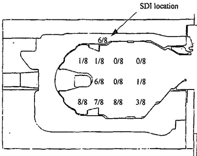
Figure 14. Laser ignition probability distribution on central plane passing through vaporiser inlet.
