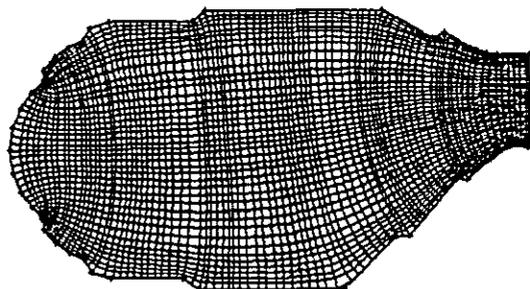
Figure 5. Combustor solution mesh in combustor plane.
