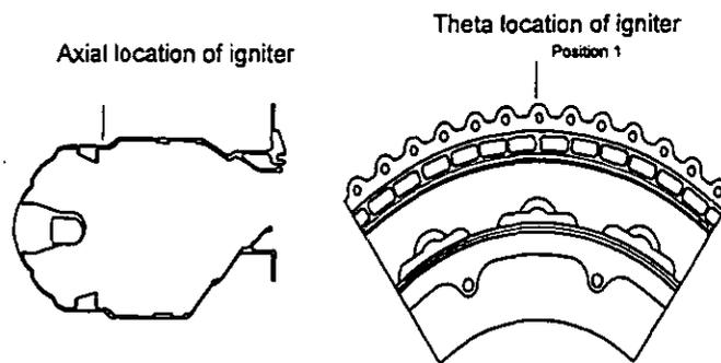
Figure 4. Surface discharge igniter location in combustor
