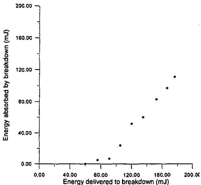
Figure 3. Variation in absorbed energy with delivered energy for a laser induced spark breakdown.
