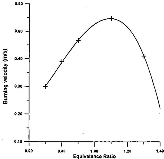
Figure 13. Variation of laminar burning velocity with equivalence ratio for a propane-air mixture at 1 atmosphere and 328 K. After Abdel-Gayed et al. [28].
