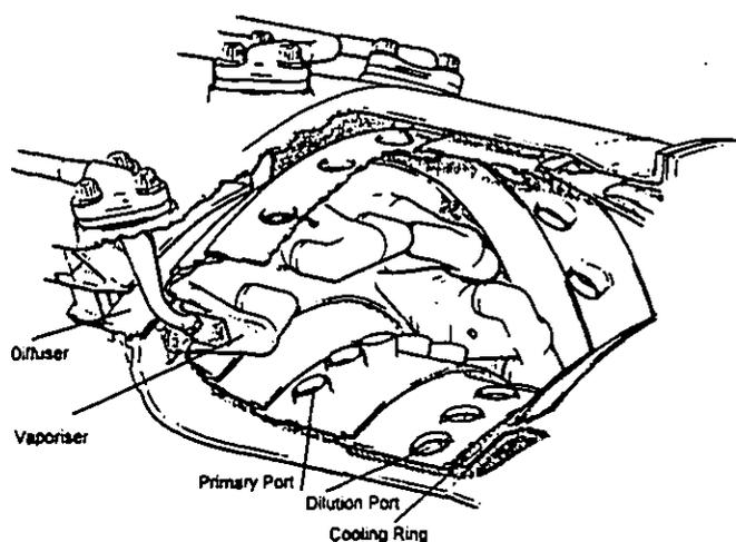
Figure 1. Pictorial view of research combustor geometry.
