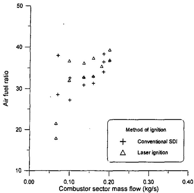
Figure 6. Comparison of  $\geq 75\%$  ignition probabilities for laser and SDI methods at the conventional SDI wall mounted location. Inlet pressure and temperature = 1.06 bar and 326 K, respectively; at an AFR of 40:1.
