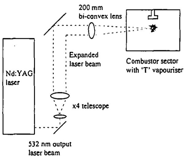
Figure 2. Laser ignition optical arrangement.
