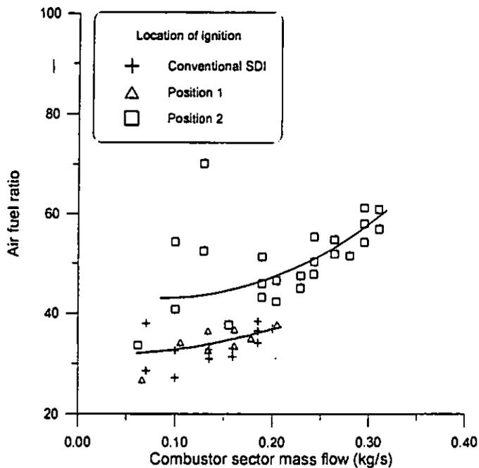
Figure 10. Comparison  $\geq 75\%$  ignition probability for laser ignition at Sites 1 and 2 and conventional SDI. Inlet pressure and temperature = 1.06 bar and 326 K, respectively; at an AFR of 40:1.
