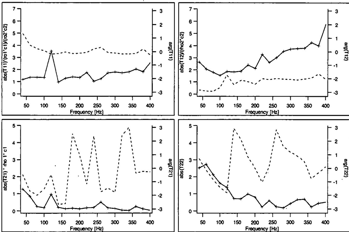
Figure 10. The transfer matrix of the burner/flame including the source term. Solid line: absolute value; dashed line: phase
