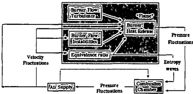
Figure 1. Noise Generation in Combustors.
