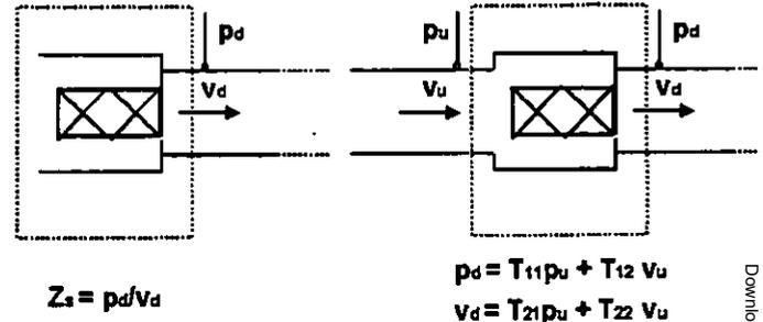
Figure 4. A burner modeled as an acoustic one-port.
