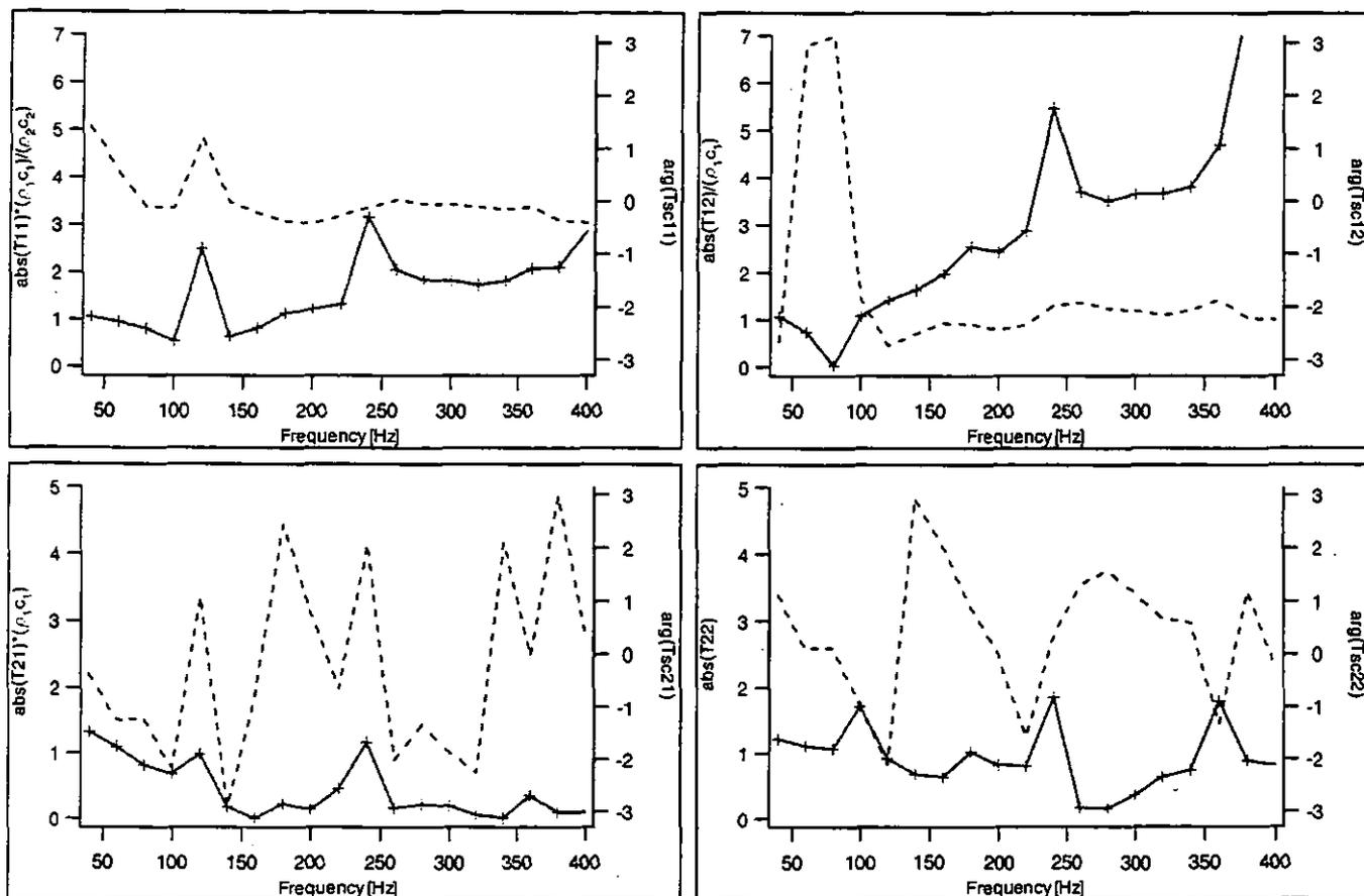
Figure 13. The transfer matrix of the flame without source term. Solid line: absolute value; dashed line: phase
