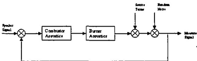
Figure 8. Different contributions to the measured signal
