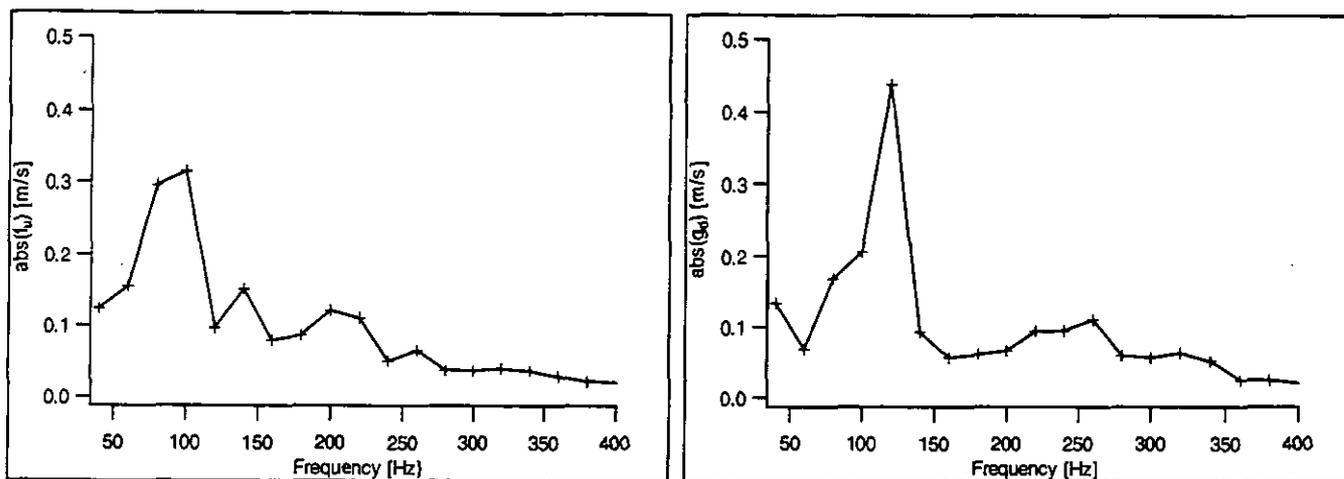
Figure 12. Incident wave components  $f_u$  (upstream of the burner) and  $g_d$  (downstream of the burner). Forcing was from upstream and downstream of the burner simultaneously.
