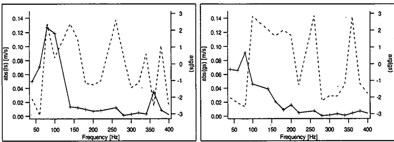
Figure 11. The source term of the flame. Solid line: absolute value; dashed line: phase
