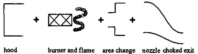
Figure 2. Example of modeling the combustor as a network of acoustic elements.
