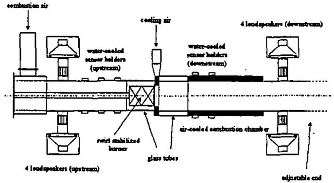
Figure 7. Experimental arrangement of the combustor.
