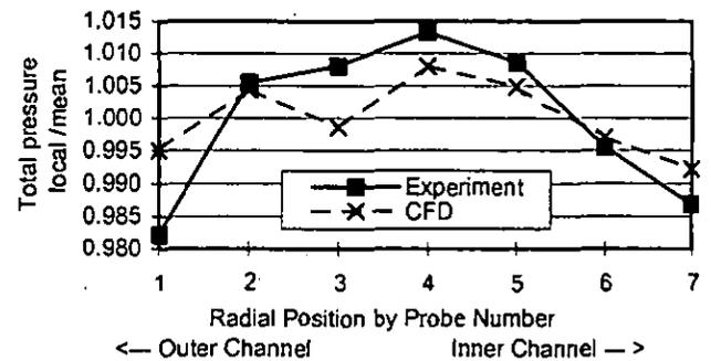
Figure 7b - Total pressure profile at the diffuser exit
