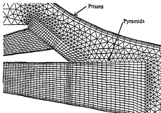
Fig. 4 - Mesh on symmetry plane of RB211-DLE model
