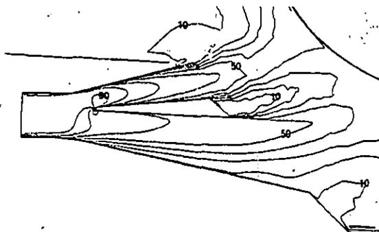
Fig. 5b - Velocity contours (increment 10 m/s) along Cut-2 of in-service diffuser
