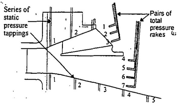
Fig. 6 - Outline of Diffuser and location of pressure probes
