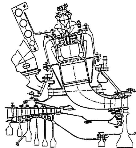
**Fig. 1 - Drawing of the RB211-DLE combustor module**
