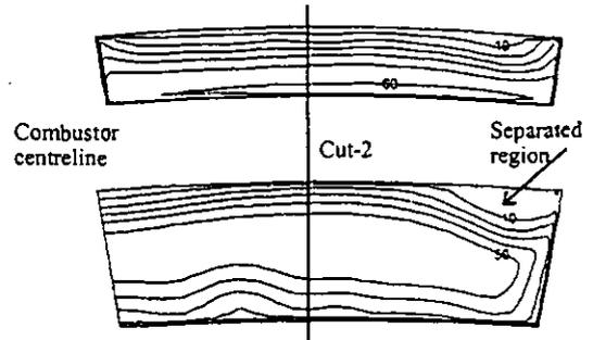
**Fig. 10h - 3D Optimum design at diffuser exit**
