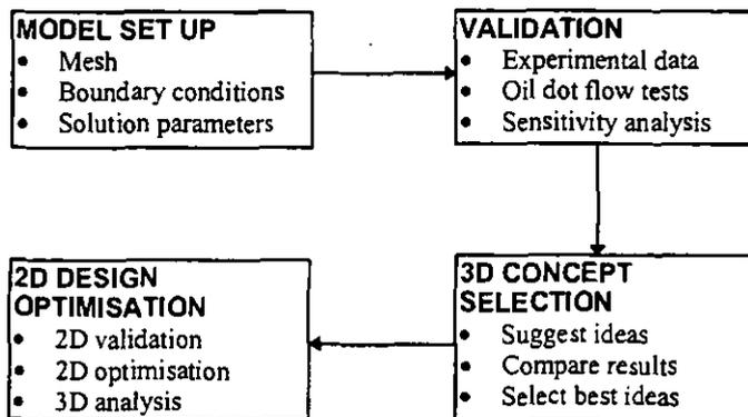
Fig. 2 - Flow diagram of design process
