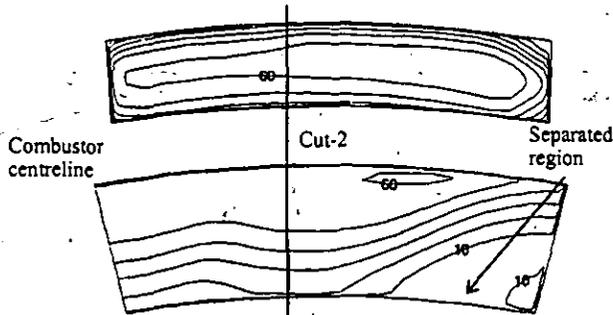
Fig. 5c - Velocity contours (increment 10m/s) at diffuser exit for the RB211-DLE CFD model
