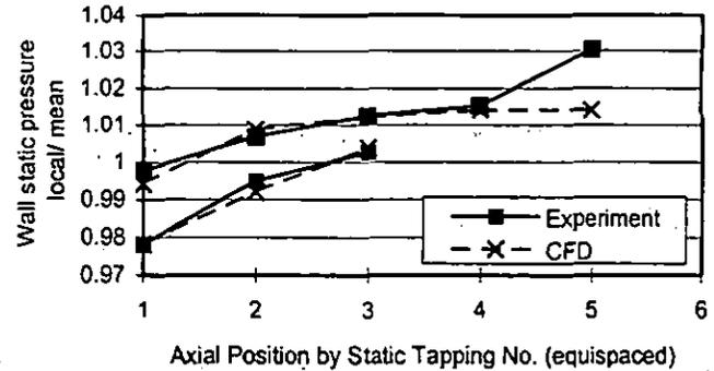
Fig. 7a - Static pressure profile on diffuser walls
