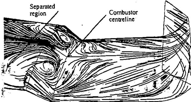
Fig. 8a - Predicted near-wall velocities on discharge nozzle
