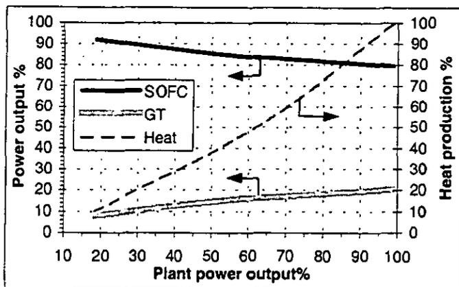
Figure 10: SOFC+GT plant power distribution and heat production as a function of the load, for constant TIT operation.
