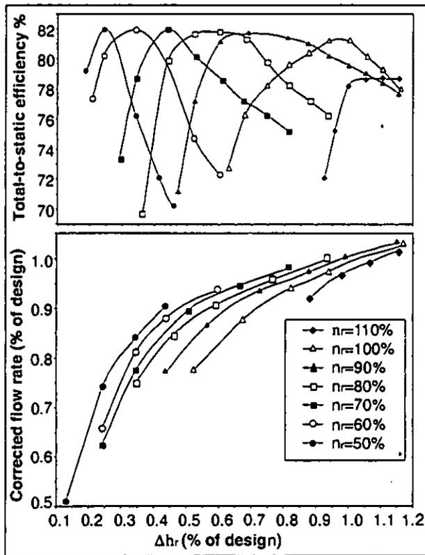
Figure 2: Characteristics of the radial turbine.
