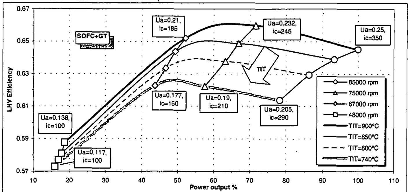
Figure 9: Partial load performances of the SOFC+GT cycle. The cell current density is reduced according to eq. 5, with lower limit at  $100 \text{ mA/cm}^2$ .
