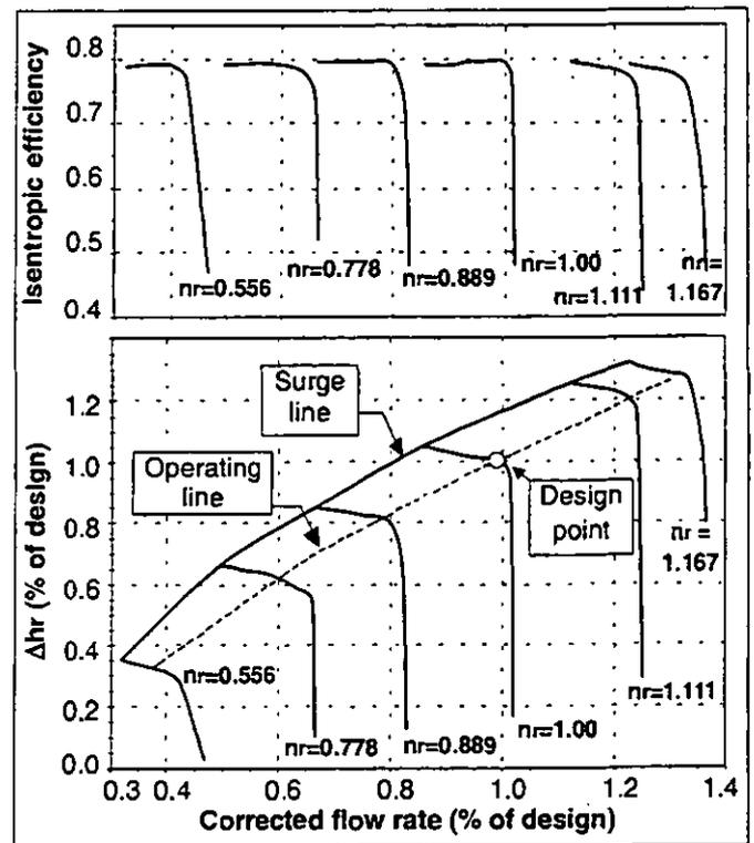
Figure 1: Characteristics of the centrifugal compressor.
