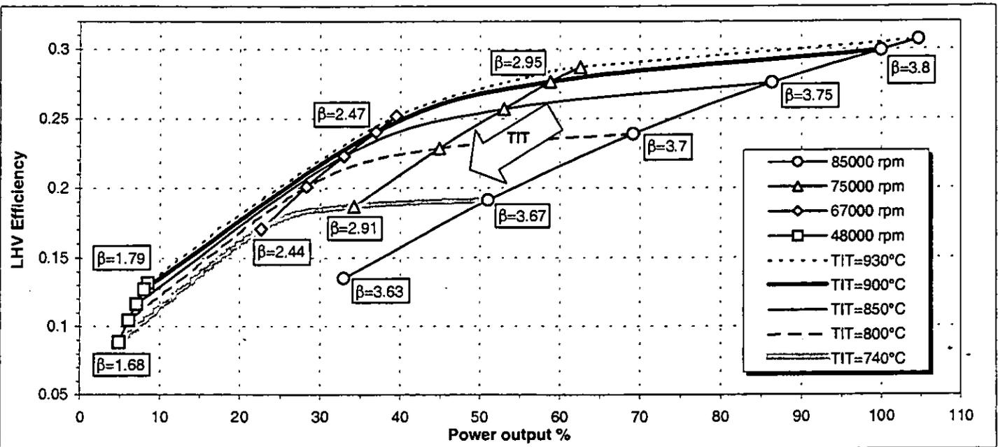
Figure 5: Calculated gas turbine performances at partial load.
