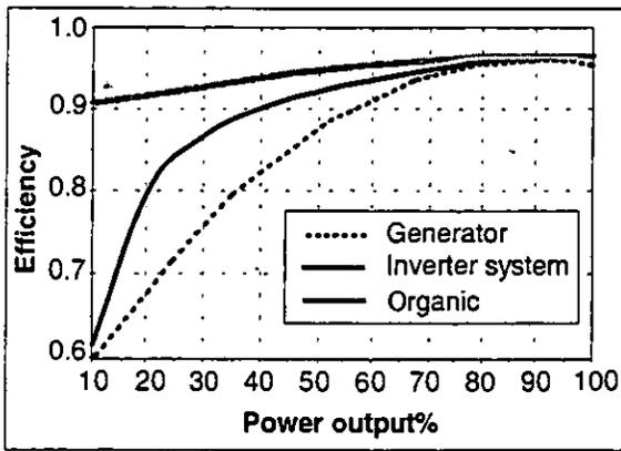
Figure 4: Electric and organic efficiencies at partial load.
