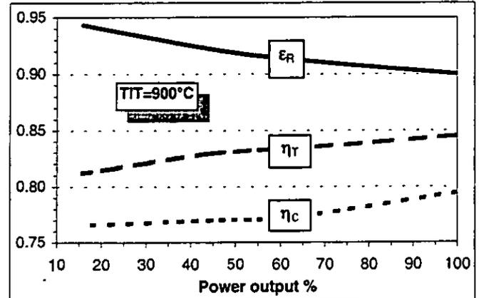
Figure 6: Compressor and turbine isentropic efficiencies and recuperator effectiveness for the gas turbine cycle at partial load (constant TIT operation).
