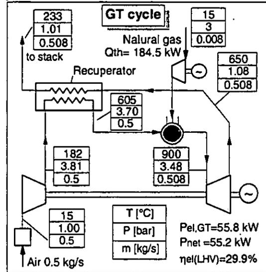
Figure 3: The recuperated gas turbine cycle.
