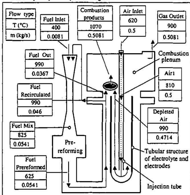
Figure 7: Tubular SOFC module configuration: spent fuel is partially recirculated and the exhaust gases of the auxiliary combustion are used to preheat the inlet air flow.
