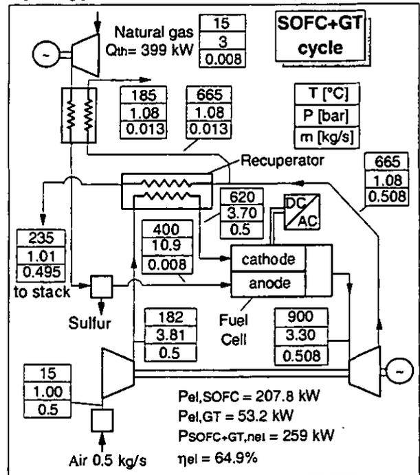
Figure 8: The recuperative SOFC+GT cycle at design conditions; components assumptions as from Tab. 1 and 2.
