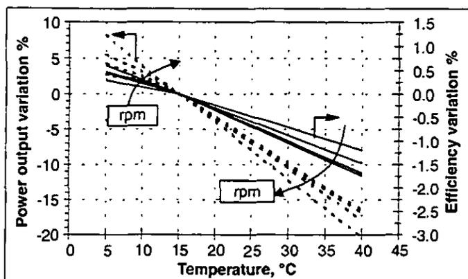
Figure 11: Effects of ambient temperature on power output (dashed line) and cycle efficiency (solid line); the TIT is set to 900°C and each group of four lines is traced for 48000, 67000, 75000 and 85000 rpm.
