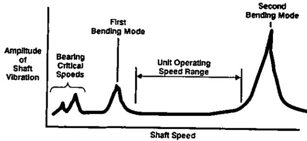
FIGURE 6. ROTORDYNAMIC RESPONSE VS SHAFT SPEED
