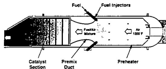
FIGURE 8. CATALYTIC COMBUSTOR DIAGRAM
