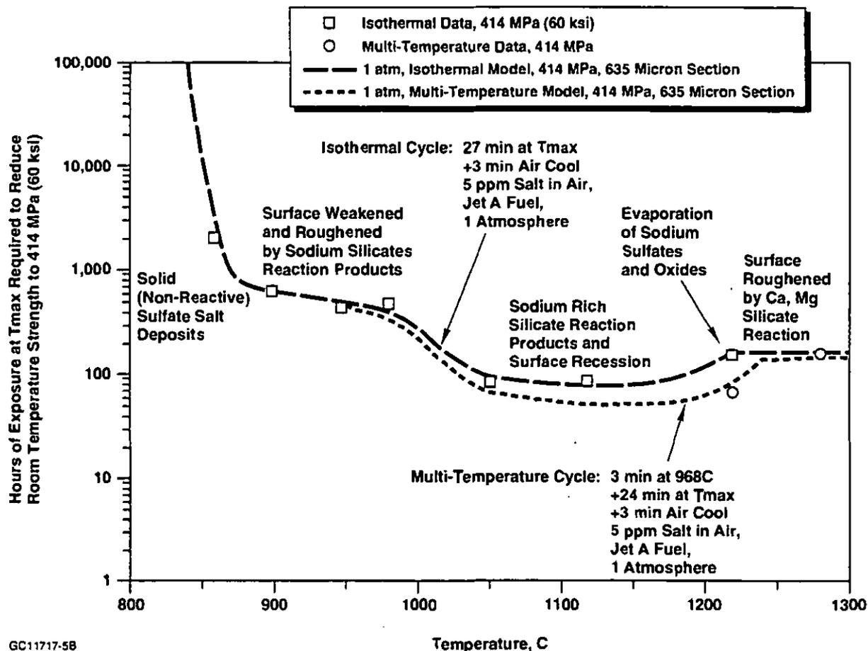
**FIGURE 5. REACTION WITH SULFATE SALT DEPOSITS FROM INGESTED SEA SALT AND FUEL CONTAMINANTS REDUCES THE STRENGTH OF NT154 SILICON NITRIDE**
