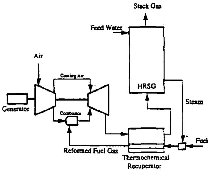
Figure 1 - Steam-TCR Cycle Diagram
