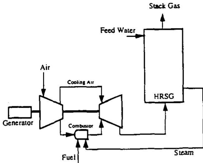
Figure 2 - Steam Injected Turbine Cycle Diagram
