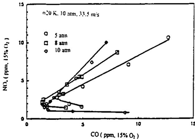
Figure 5. Experimental CO and NO<sub>x</sub> data of Lovett and Mick (1995) shown on an emissions tradeoff plot. On this type of graph NO<sub>x</sub> ~  $\phi$ . Regions of kinetic and equilibrium CO (see Fig. 4) are apparent. The operating conditions shown in the upper left hand corner of the graph should read "620 K, 33.5 m/s"; "10 atm" is a typographical error.
