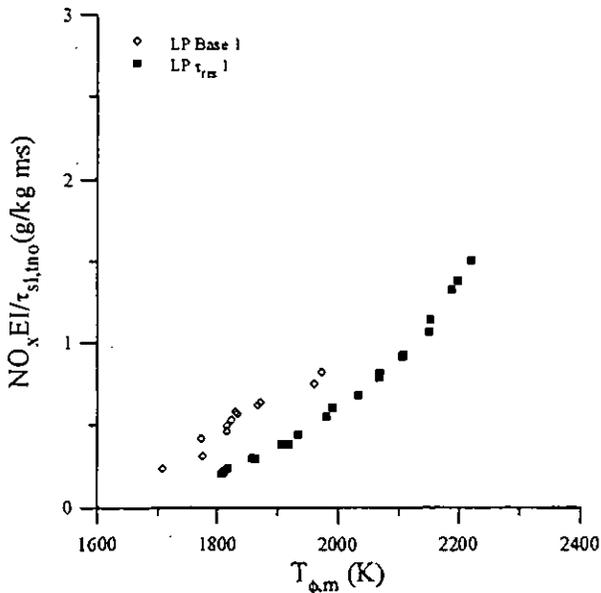
Figure 1. Graph of Combustor A LP  $\text{NO}_x$  data divided by corresponding  $\text{NO}_x$  fluid mechanic times ( $\tau_{sl,tno}$ ). The open diamonds represent data obtained at a longer residence time than the closed squares. Inlet temperature and pressure are constant. The fact that the curves do not collapse indicates that unmixedness ( $s$ ) is a variable between the two datum sets.
