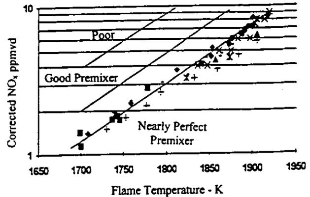
Figure 3. Schematic showing the best fit through the Leonard and Stegmaier (1994) data. The Leonard and Stegmaier best fit is used as the perfectly premixed ( $s = 0$ ) baseline in this case. The other two other example trendlines correspond to experimental data with  $s$  greater than zero (from Leonard and Stegmaier, 1994).
