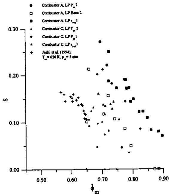
Figure 9. Unmixedness levels deduced from CO emissions (Eq. 6) for the 620 K, 5 atm tests of Joshi et al. (1994) shown in Fig. 7 and for selected Combustor A and C (see text) operating conditions (from Mello et al., 1997).
