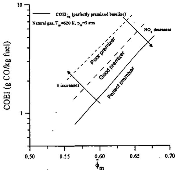
Figure 10. Expected trends in measured COEI with  $s$  for mean equivalence ratio greater than  $\phi^*$ . The baseline case corresponds to equilibrium at  $s = 0$ .
