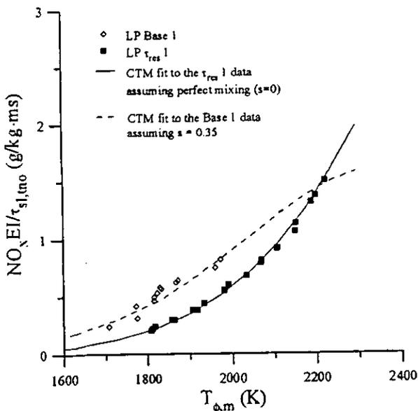
Figure 2. Using the best fit through the LP  $\tau_{res 1}$  data for the perfectly premixed baseline in Eq. (1),  $s$  is adjusted such that the LP  $\tau_{res 1}$  best fit correlates the LP Base 1 data. The value of  $s$  corresponding to the LP Base 1 data is estimated to be 0.35.
