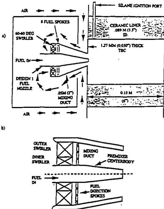
Figure 6. a) Single cup test combustor cross section; b) DACRS II premixer cross section (Joshi et al., 1994).
