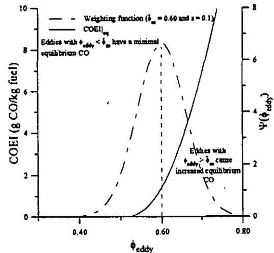
Figure 8. Graph indicating the relationship between a typical Gaussian eddy equivalence ratio distribution and the equilibrium CO curve for the inlet conditions of the data in Fig. 7.
