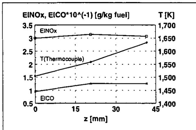
Fig. 16  $\text{NO}_x$ ,  $\text{CO}$  emission index and temperature at the exit of the combustor at  $y = 0$  mm and several  $z$ -positions
