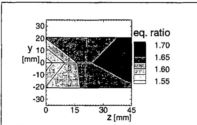
Fig. 5 Equivalence ratio at the exit of the primary zone
