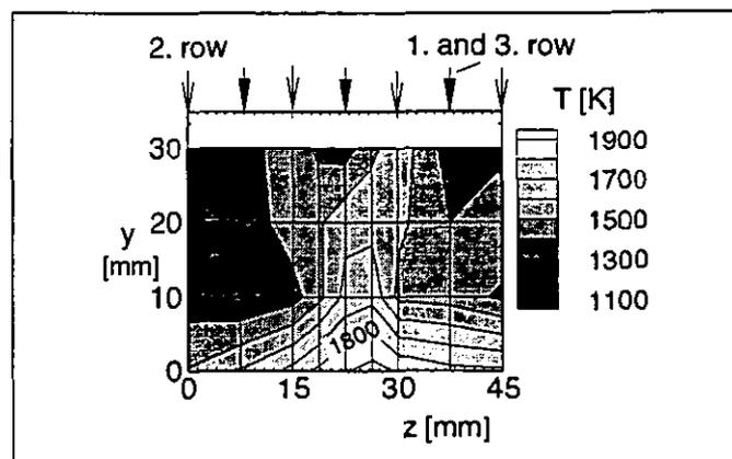
Fig. 14 Mean temperature at the exit of the quench zone
