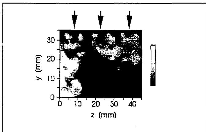
Fig. 12 Distribution of OH radicals in a cross-section through the first row of secondary air holes ( $x = 100$  mm)
