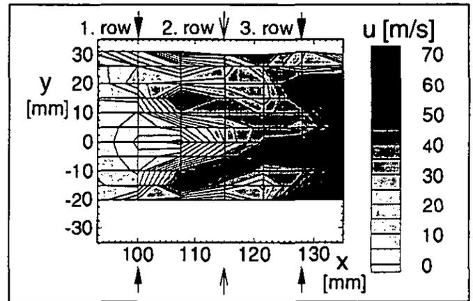
Fig. 6 Axial velocity in the cross-section  $z = 22.5$  mm
