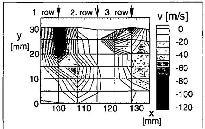
Fig. 7 Vertical velocity in the cross-section  $z = 22.5$  mm
