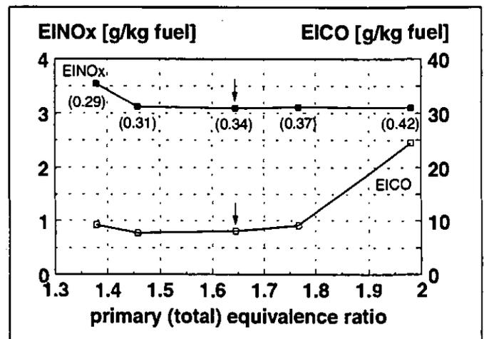
Fig. 17 Emission index of  $\text{NO}_x$  and  $\text{CO}$  at the exit of the combustor (mass averaged values)
