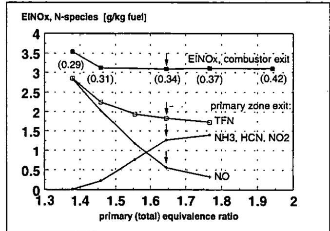
Fig. 3  $\text{EINO}_x$  at the combustor exit and N-species at the exit of the primary zone (mass averaged values)
