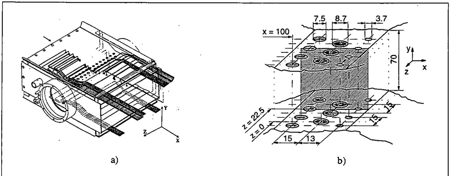
Fig. 2 Perspective view of the liner a) and the quench zone geometry b)
