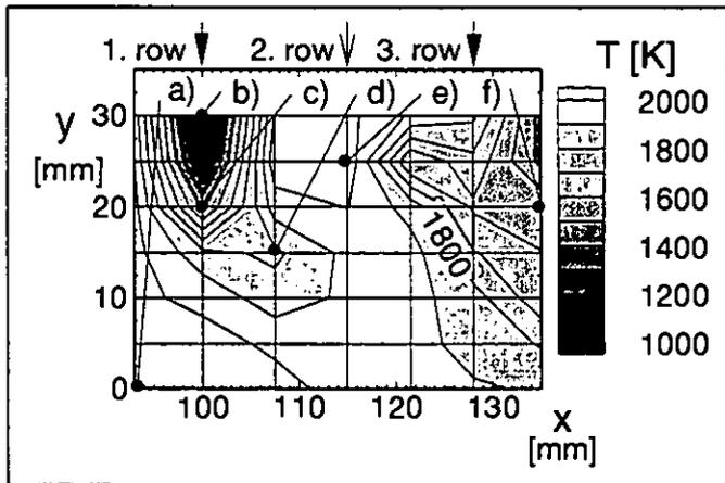
Fig. 9 Mean temperature in the cross-section  $z = 22.5$  mm
