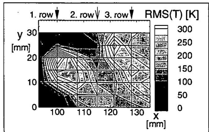
Fig. 11 RMS temperature in the cross-section  $z = 22.5$  mm
