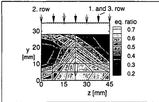
Fig. 15 Equivalence ratio at the exit of the quench zone
