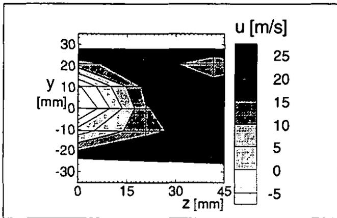
Fig. 4 Axial velocity at the exit of the primary zone
