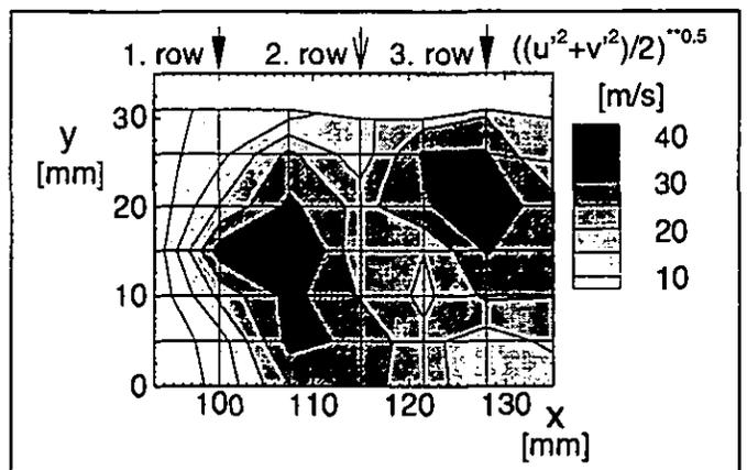
Fig. 8 RMS velocity in the cross-section  $z = 22.5$  mm
