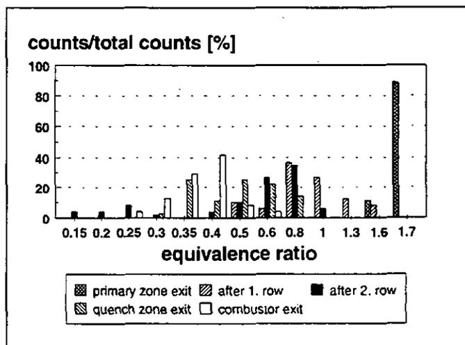
Fig. 13 Histograms of the equivalence ratio in cross-sections at five different axial positions
