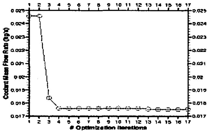
Figure 15. Evolution of coolant mass flow rate for the minimization of coolant ejection temperature using the maximum temperature equality constraint.
