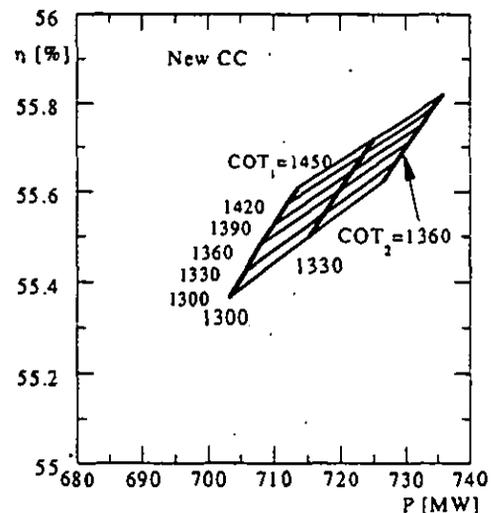
Fig. 5  $\eta$  versus  $P$  for different  $COT_1$  and  $COT_2$  values. (case of the new CC)
