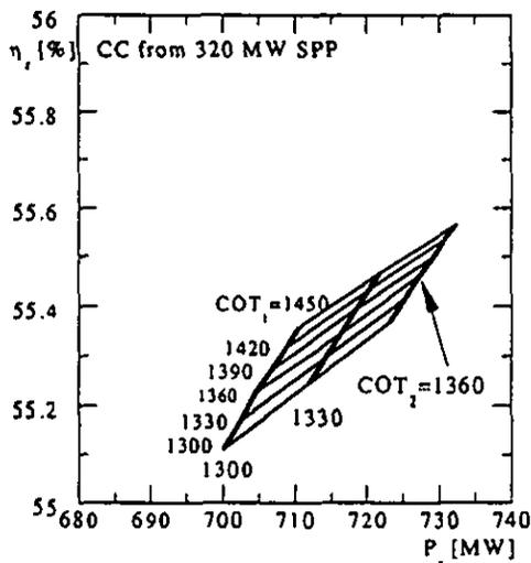
Fig. 4  $\eta$ , versus  $P$ , for different  $COT_1$  and  $COT_2$  values. (case of the CC derived from 320 MW SPP)
