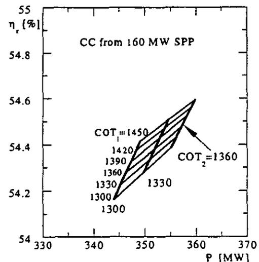
Fig.3  $\eta_r$  versus  $P_r$  for different  $COT_1$  and  $COT_2$  values. (case of the CC derived from 160 MW SPP)
