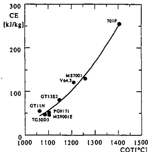
Fig.2 CE versus COT for some Brayton cycle gas turbines
