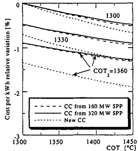
Fig.6 Cost per kWh relative variation [%] versus COT<sub>1</sub> for different COT<sub>2</sub> values
