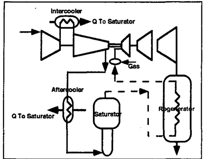
Fig. 6 - Simplified HAT cycle schematic
