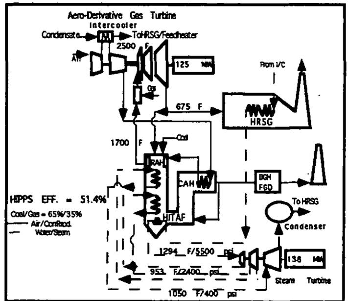
Fig. 4 - HIPPS/ICAD with advanced steam turbine technology
