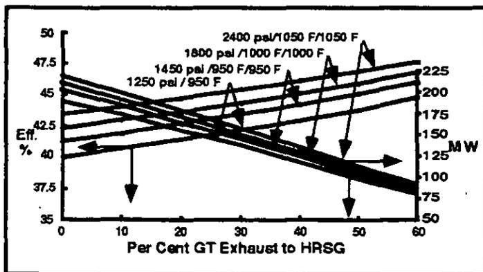
Fig. 10 - Results of Repowering Parametric Study
