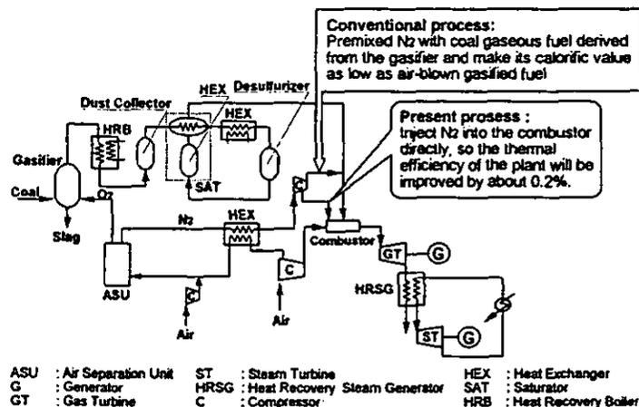
Fig.1 Schematic diagram of oxygen-blown IGCC system
