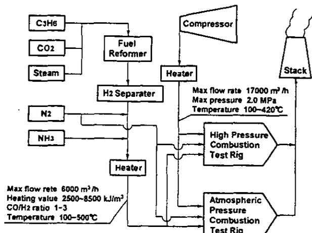
Fig.9 Schematic diagram of experimental facility
