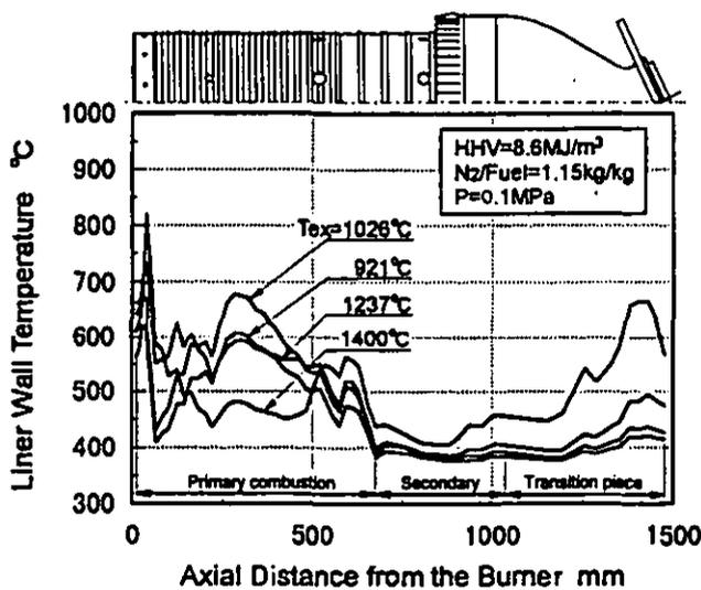
Fig.11 Combustor wall temperature distribution using the average gas temperature of combustor outlet as a parameter
