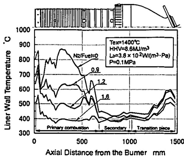
Fig.12 Effect of the nitrogen injection flow rate from the burner on the combustor wall temperature distribution.
