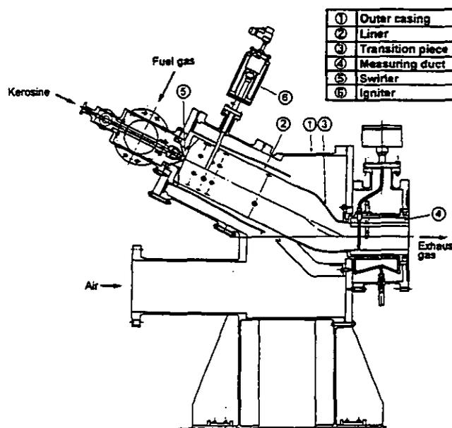
Fig.10 Atmospheric pressure combustion test rig
