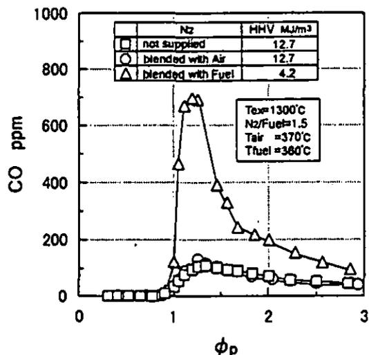
Fig.7 Effect of nitrogen injection on CO emission characteristics in two-staged combustion, using a small diffusion burner
