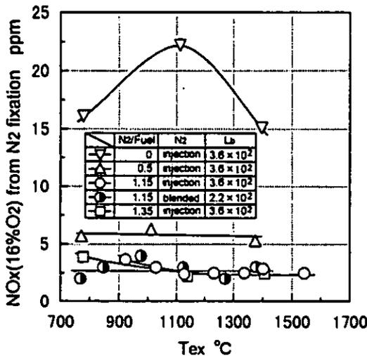
Fig.16 Effect of the combustor outlet gas temperature on NOx emission concentration from nitrogen fixation
