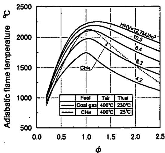
Fig.2 Relationship between equivalence ratio and adiabatic flame temperature for coal gas and CH<sub>4</sub>
