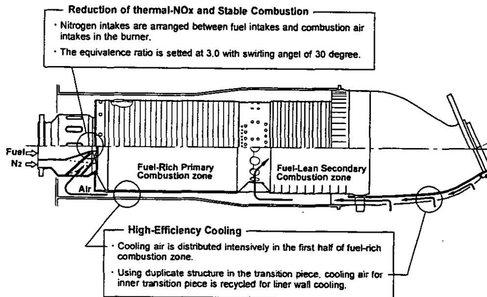
Fig.4 Design concept of a medium-Btu fueled gas turbine combustion
