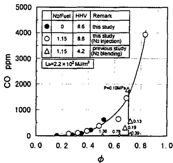
Fig.14 Effect of the nitrogen injection on CO emission characteristics
