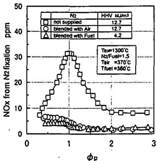
Fig.6 Effect of nitrogen injection on NO<sub>x</sub> emission characteristics in two-staged combustion, using a small diffusion burner
