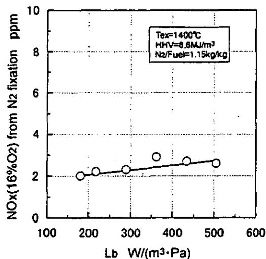
Fig.15 Effect of the combustor loading rate on NOx emission concentration from nitrogen fixation
