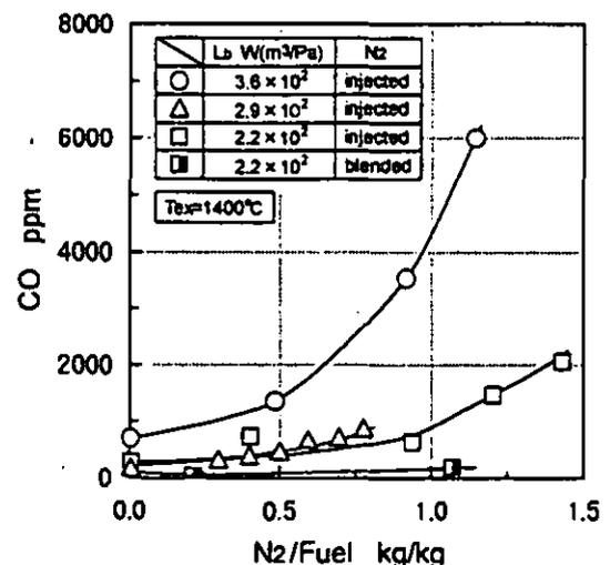
Fig.13 Effect of the loading rate in the combustor on CO emission characteristics
