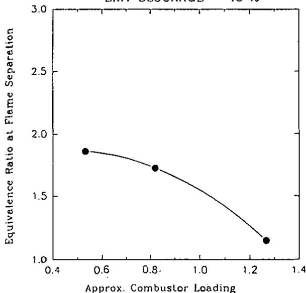
Fig. 10 Influence of Combustor Loading on Equivalence Ratio for Flame Separation at 45 Percent Exit Blockage
