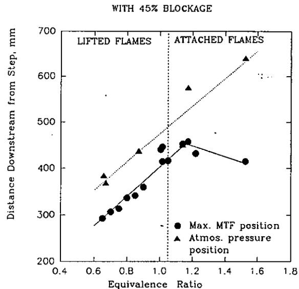
Fig. 24 Downstream Positions Where Atmospheric Pressure and Maximum Normalized Wall Temperature Are Attained as Equivalence Ratio Is Varied for Fixed Exit Blockage
