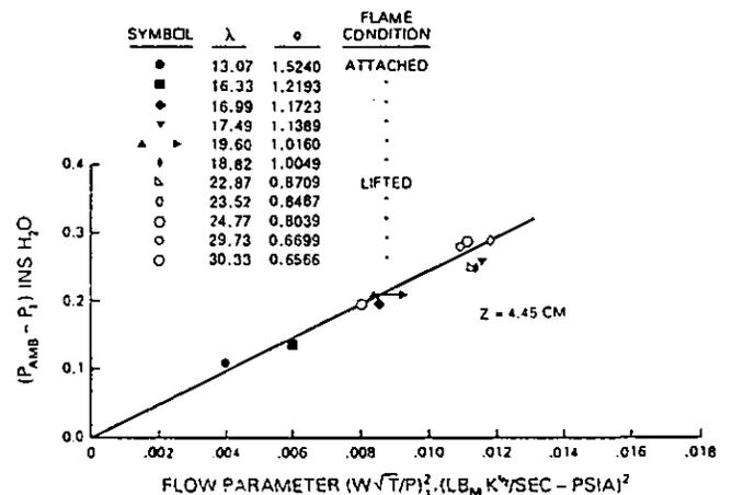
Fig. 21 Suppression of Dependency of Wall Static Pressure on Jet Velocity Ratio by Combustion with a Free Exit
