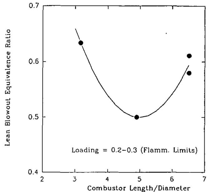
Fig. 12 Dependence of Lean Blowout at Low Loadings on Combustor Length with 45 Percent Exit Blockage
