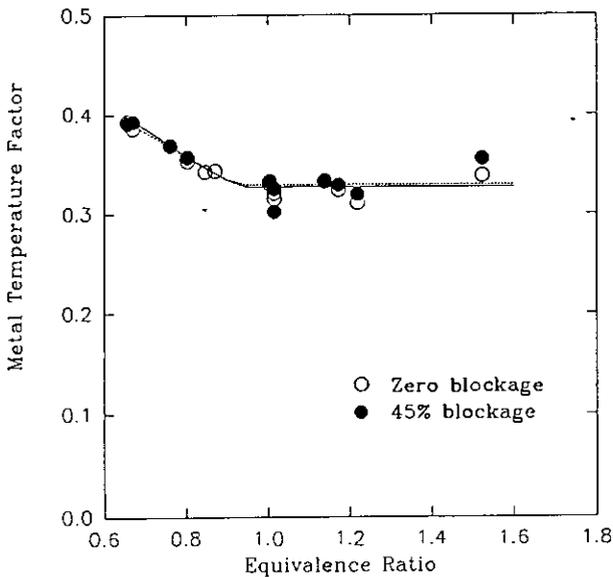
Fig. 15 Normalized Wall Temperatures at 126 mm from Step-Plane for Zero and 45 Percent Exit Blockage, Showing Influence of Equivalence Ratio
