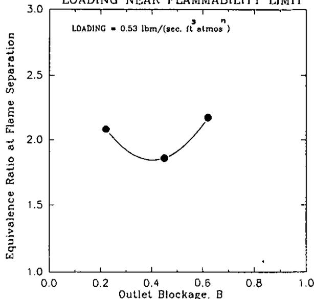
Fig. 9 Dependence of Equivalence Ratio for Flame Separation on Exit Blockage for Low Combustor Loading
