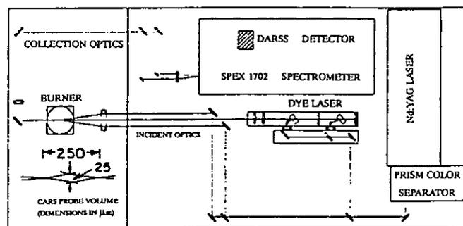
Fig. 2 Arrangement of the CARS System Optics
