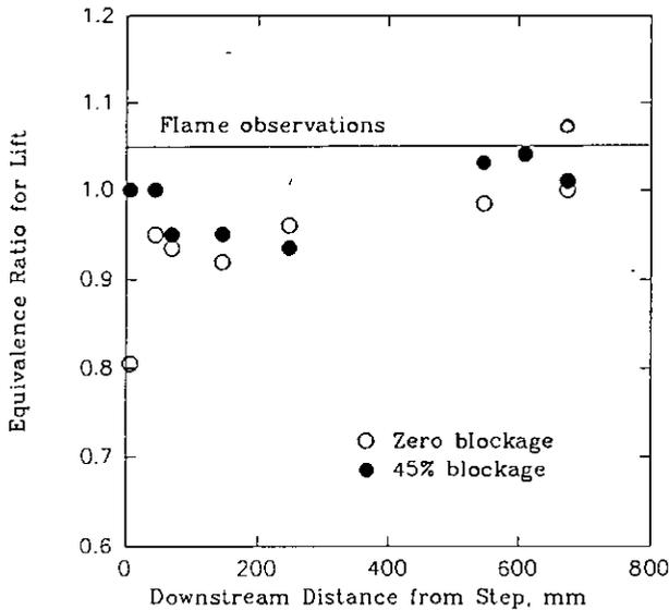
Fig. 16 Indicated Equivalence Ratios for Flame-Lift from Wall Temperatures, Compared with Direct Observations
