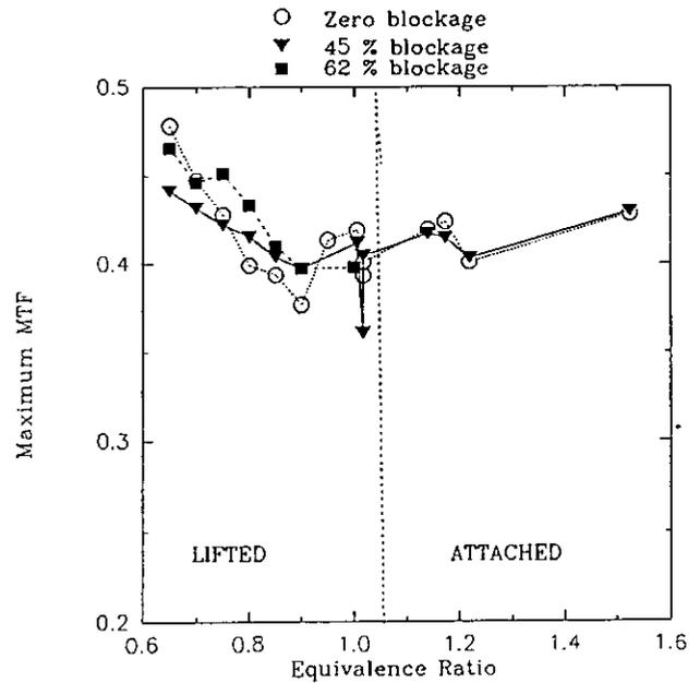
Fig. 17 Variations of Maximum Normalized Wall Temperatures for Lifted and Attached Flames at Several Values of Exit Blockage
