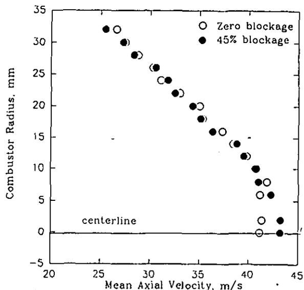
Fig. 4 Radial Profiles of Mean Axial Velocity in Isothermal Flow at 300 mm Downstream from the Step-Plane, Showing Central Flow Net Acceleration with Exit Blockage
