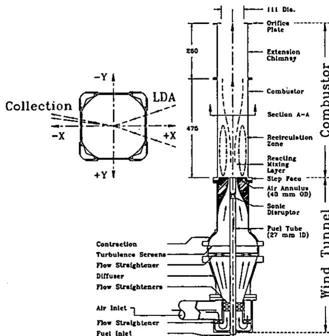
Fig. 1 Research Combustor, Showing Axes Convention
