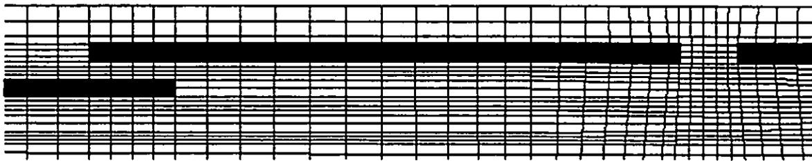
Figure 5. Close-up of Part of the Outer Liner Grid with Wall Cells Shaded
