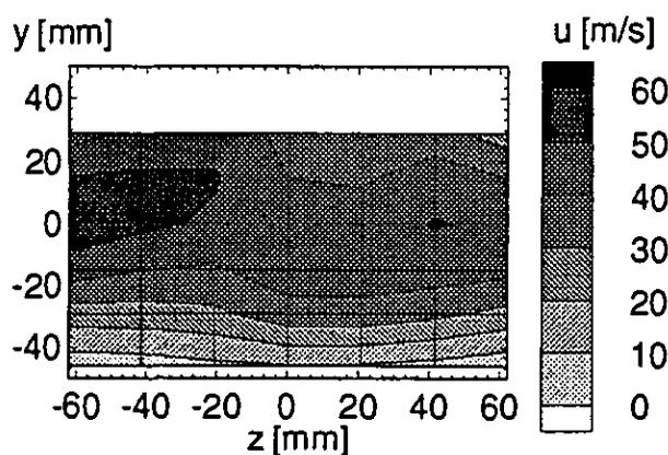
Fig. 11 Measured Distribution of the Axial Velocity Component in
