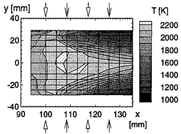
Fig. 17 Measured Temperature Distributions in Axial-Vertical Edge-Plane ( $z=-38\text{mm}$ )
