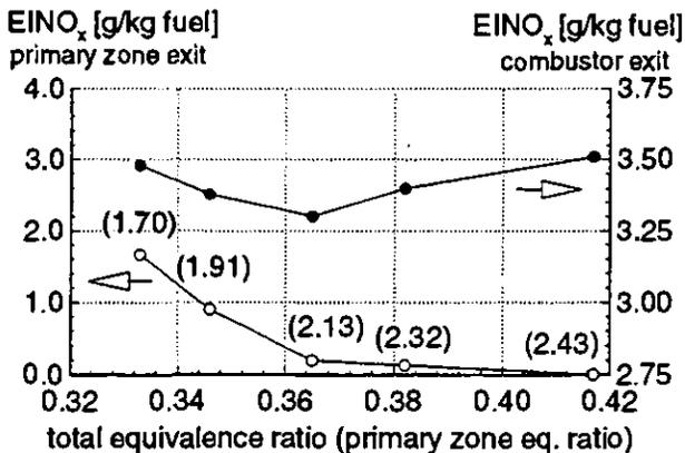
Fig. 4 EINO<sub>x</sub> as a Funktion of the Total resp. the Primary Zone Equivalence Ratio
