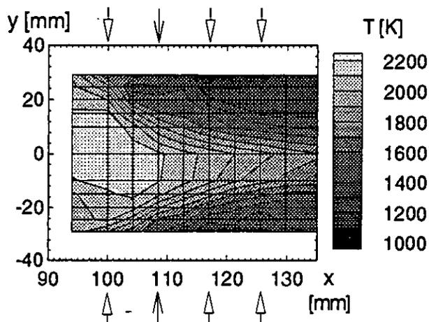
Fig. 16 Measured Temperature Distributions in Axial-Vertical Mid-Plane ( $z=-4\text{mm}$ )
