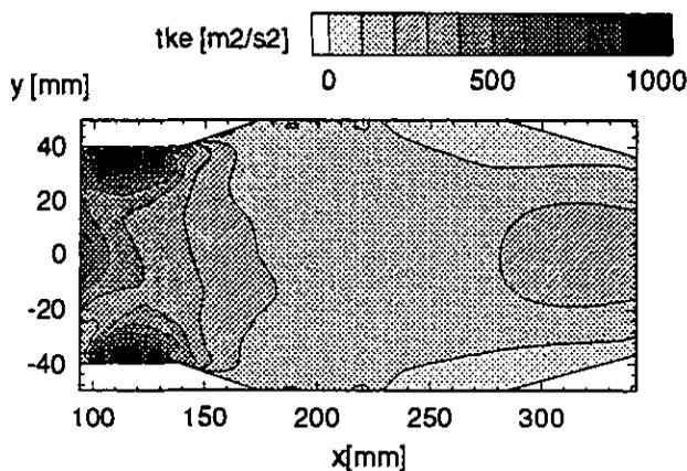
Fig. 10 Distribution of the Turbulent Energy in Axial-Vertical Midplane ( $z = -4$  mm)
