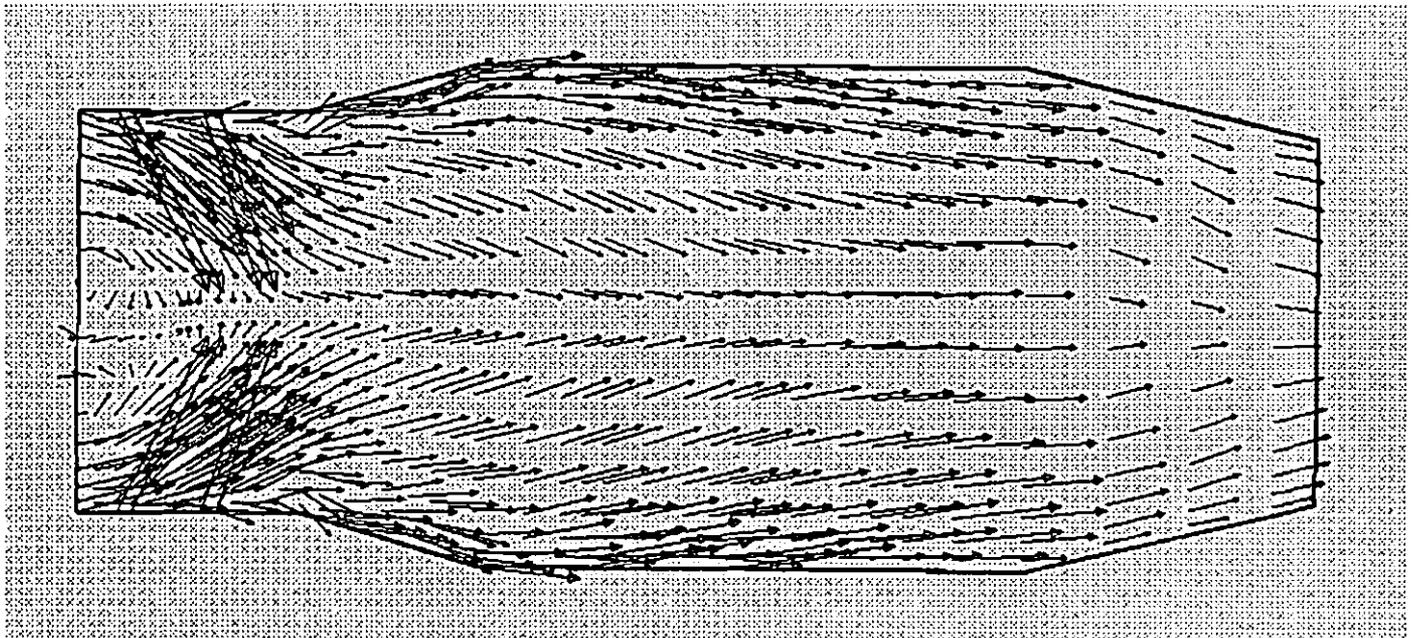
Fig. 7 Flow Vectors in Axial-Vertical Midplane ( $z=-4$  mm)
