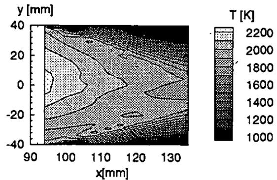
Fig. 9 Calculated Temperature Distributions in Axial-Vertical Edge-Plane ( $z=-38$ mm)
