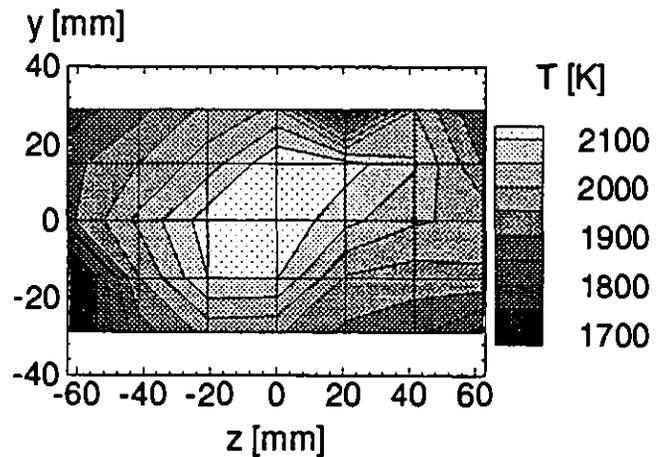
Fig. 6 Measured Temperature Distribution at Primary zone Exit
