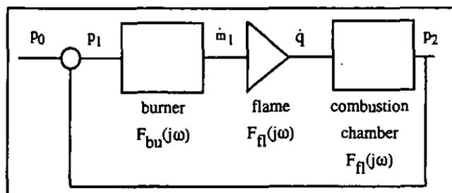
FIG. 1: Oscillating Circuit of a Combustor System
