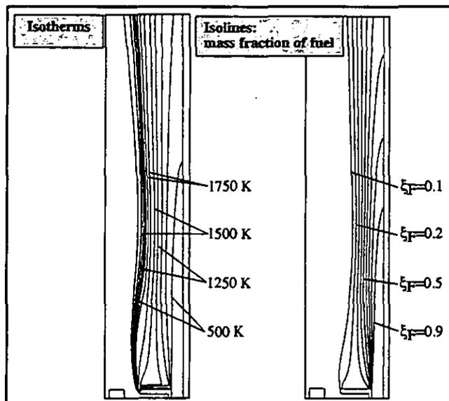
FIG.9: BAFFLE-PLATE-STABILIZED BURNER: STEADY-STATE-CALCULATION
