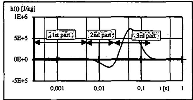
FIG. 12: UNIT FUNCTION OF THE TURBULENT DIFFUSION FLAME
