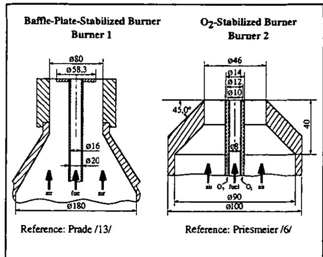
FIG. 4: BURNER CONFIGURATIONS
