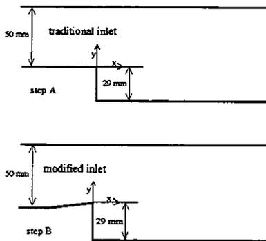
Fig. 2 Configurations of the traditional and the modified inlets of the sudden expansion combustor.
