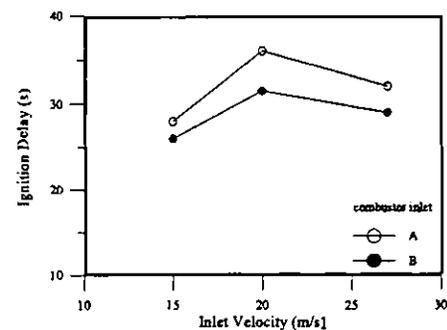
Fig. 15 Effects of inlet velocity of the flow on the ignition delay at oxygen concentration of 15%. (uncertainty in ignition delay is less than  $\pm 7.3\%$ )
