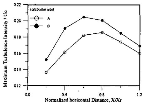
Fig. 10 Maximum turbulence intensities at various cross sections of the two different combustors. (uncertainty in turbulence intensity is less than  $\pm 4.9\%$ )
