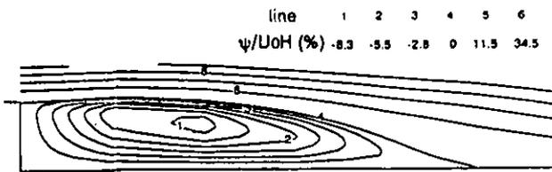
Fig. 7 Streamlines of the flow field in the traditional combustor. (uncertainty in mean horizontal velocity is less than  $\pm 3.2\%$ )
