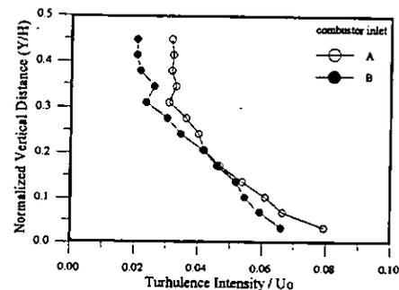
Fig. 5 Distributions of the turbulence intensity at the inlets (A) traditional, (B) modified. (uncertainty in turbulence intensity is less than  $\pm 4.9\%$ )
