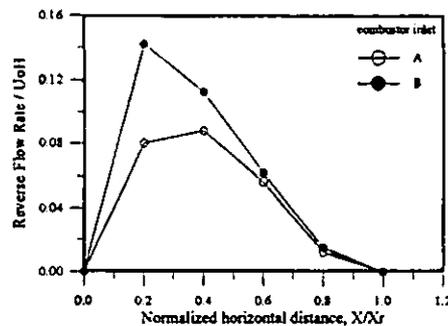
Fig. 9 Dimensionless reverse flow rates at various cross sections of the two different combustors. (uncertainty in dimensionless reverse flow rate is less than  $\pm 3.2\%$ )
