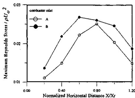
Fig. 11 Maximum Reynolds stresses at various cross sections of the two different combustors. (uncertainty in Reynolds stress is less than  $\pm 13\%$ )
