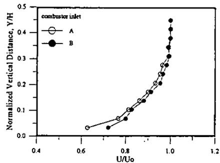
Fig. 3 Distributions of the horizontal velocity at the inlets (A) traditional, (B) modified. (uncertainty in mean horizontal velocity is less than  $\pm 3.2\%$ )
