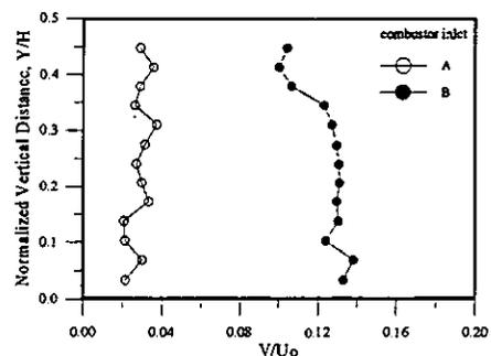
Fig. 4 Distributions of the vertical velocity at the inlets (A) traditional, (B) modified. (uncertainty in dimensionless reverse flow rate is less than  $\pm 3.2\%$ )
