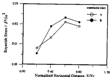
Fig. 13 Comparisons of the Reynolds stress along the dividing streamlines of the recirculation zone of the two different combustors. (A) traditional, (B) modified. (uncertainty in Reynolds stress is less than  $\pm 13\%$ )
