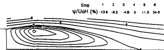
Fig. 8 streamlines of the flow field in the modified combustor. (uncertainty in mean horizontal velocity is less than  $\pm 3.2\%$ )
