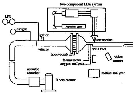
Fig. 1 A schematic diagram of the experimental apparatus.
