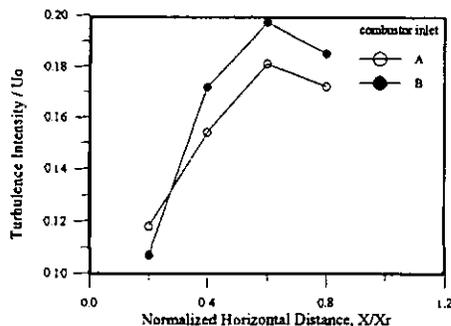
Fig. 12 Comparisons of the turbulence intensities along the dividing streamlines of the recirculation zone of the two different combustors. (A) traditional, (B) modified. (uncertainty in turbulence intensity is less than  $\pm 4.9\%$ )
