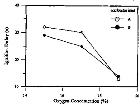
Fig. 14 Effects of oxygen content of the flow on the ignition delay at  $U_0 = 15$  m/s. (uncertainty in ignition delay is less than  $\pm 7.3\%$ )
