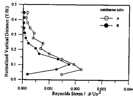
Fig. 6 Distributions of the Reynolds stress at the inlets (A) traditional, (B) modified. (uncertainty in Reynolds stress is less than  $\pm 13\%$ )
