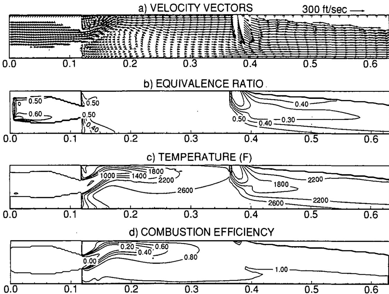
FIGURE 4. PREDICTED KEY FLOW FIELD PARAMETERS FOR DRY LOW  $\text{NO}_x$  CONFIGURATION 2.
