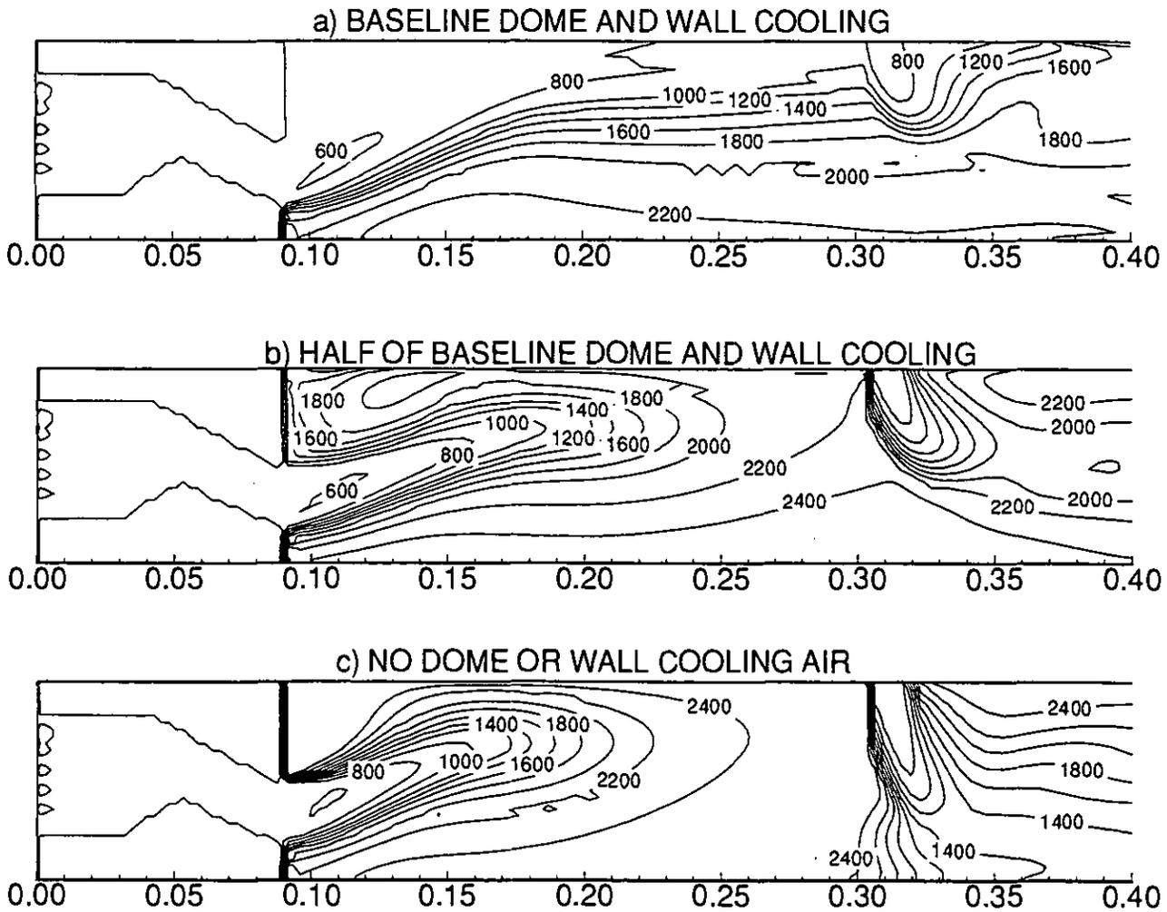
FIGURE 5. PREDICTED EFFECT OF WALL COOLING ON COMBUSTOR TEMPERATURE DISTRIBUTION.
