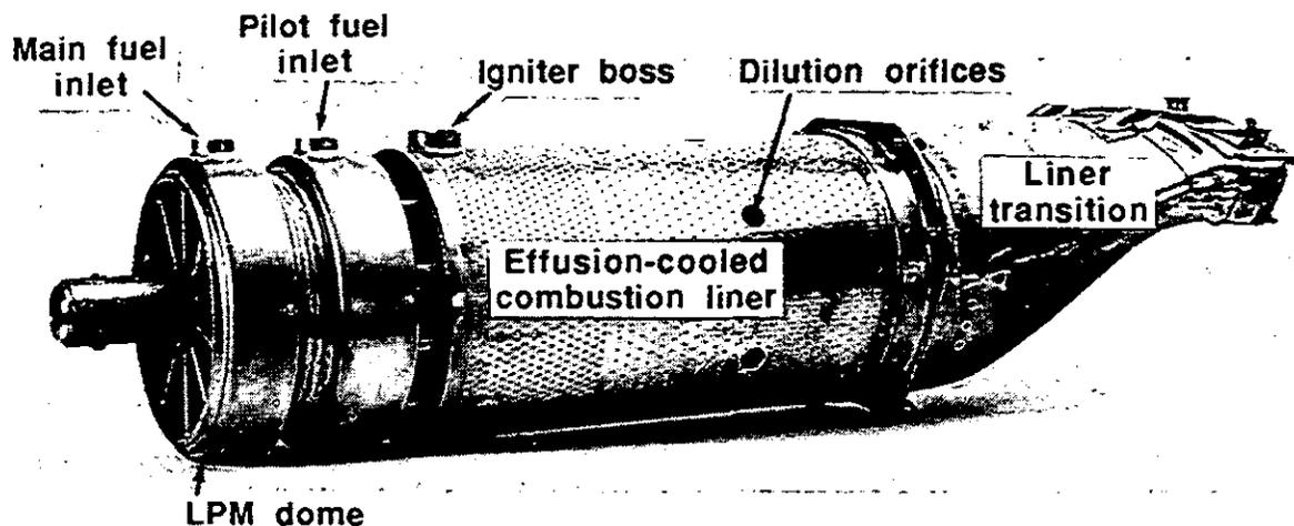
FIGURE 3. PHOTOGRAPH OF DRY LOW  $\text{NO}_x$  COMBUSTOR ASSEMBLY.
