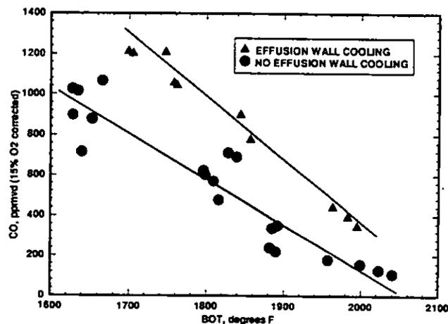
FIGURE 15. EFFECT OF WALL COOLING ON CO EMISSIONS.
