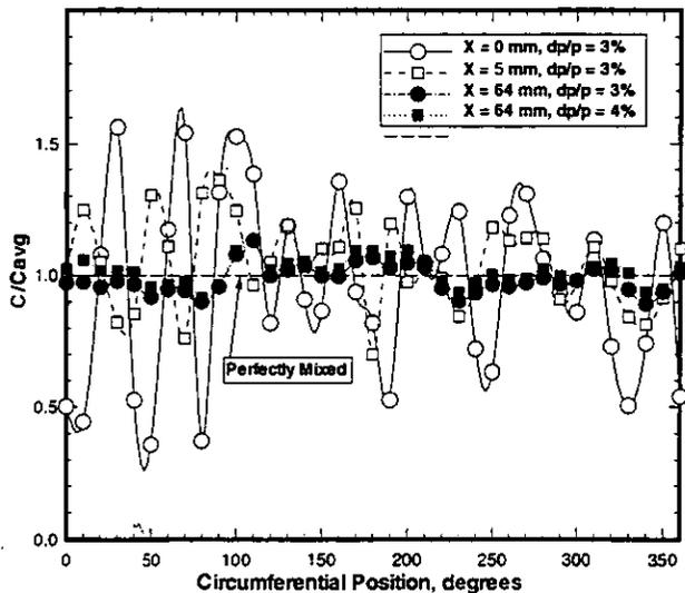
FIGURE 8. MEASURED FUEL/AIR MIXING CHARACTERISTICS IN CONFIGURATION 1 LPM DOME.
