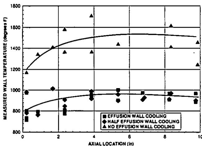
FIGURE 20. MEASURED WALL TEMPERATURE FOR DIFFERENT LINER WALL COOLING FLOW RATES.
