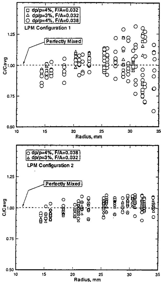
FIGURE 9. MEASURED FUEL/AIR MIXING PERFORMANCE OF DRY LOW  $NO_x$  CONFIGURATIONS 1 AND 2.
