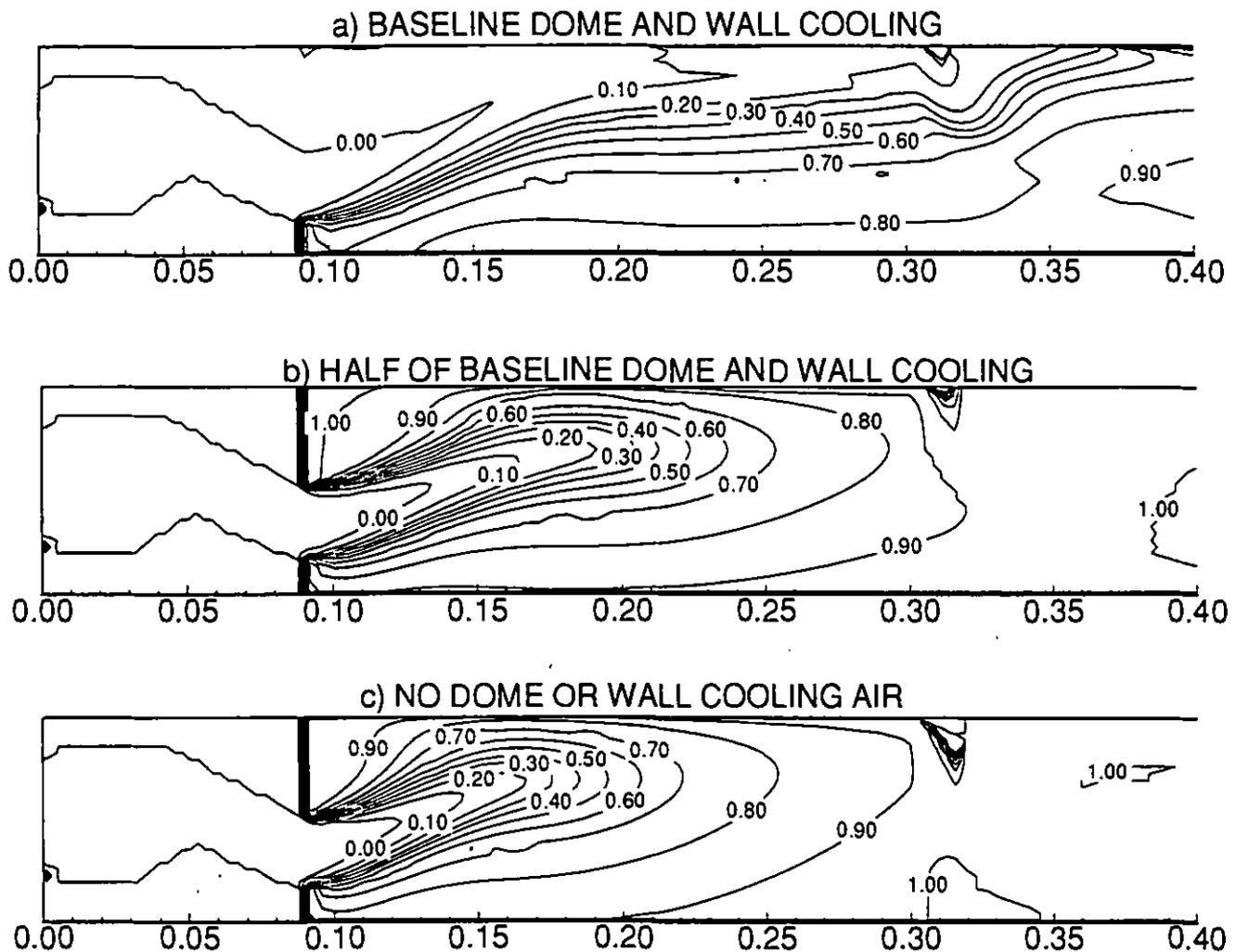
FIGURE 6. PREDICTED EFFECT OF WALL COOLING ON COMBUSTION EFFICIENCY.
