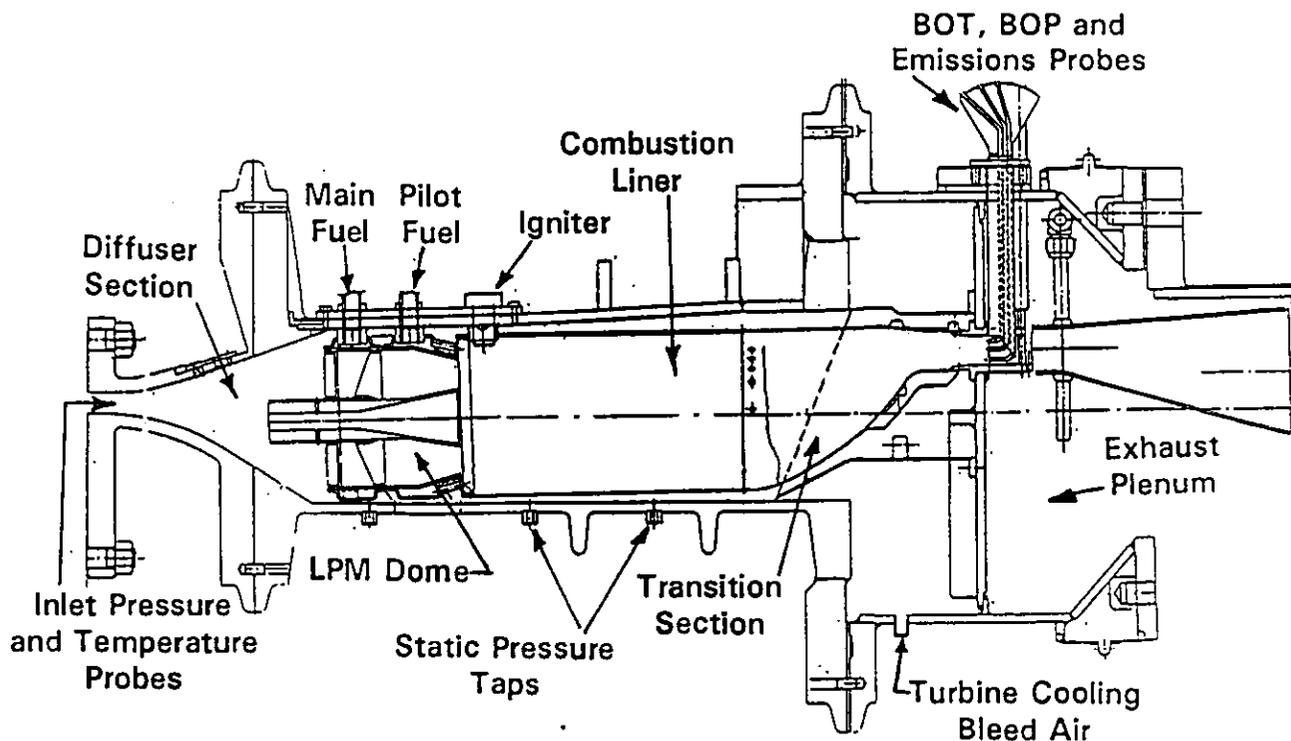
FIGURE 11. SCHEMATIC OF RIG TEST FACILITY.
