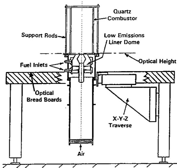
FIGURE 7. SCHEMATIC OF BENCH TEST FACILITY.
