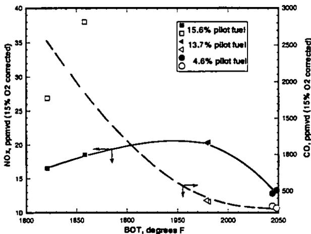
FIGURE 14. EMISSIONS RESULTS OF PILOT SUPPORTED ULTRA-LEAN COMBUSTION IN CONFIGURATION 2.
