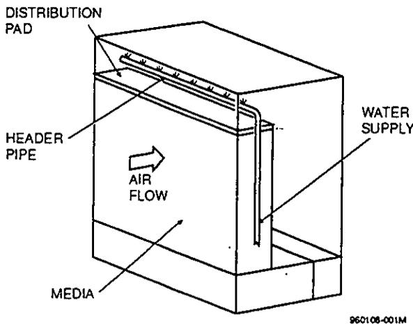
Figure 1. Evaporative Cooler
