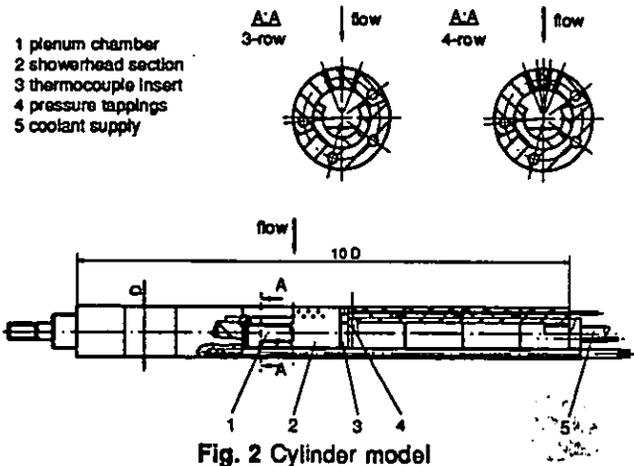
Fig. 2 Cylinder model
