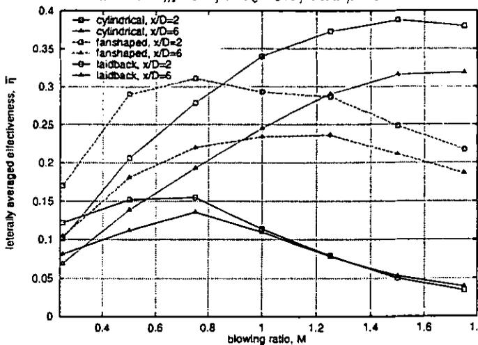
FIG. 9: Effect of blowing ratio  $M$  on laterally averaged effectiveness  $\bar{\eta}$  for the three holes tested at  $Ma_m=0.6$ ,  $Ma_c=0.0$ ,  $\beta=0^\circ$
