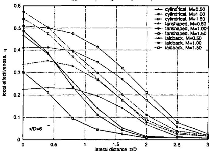
FIG. 6: Local lateral effectiveness  $\eta$  for the three holes tested at  $Ma_m=0.6$ ,  $Ma_c=0.0$ , and  $\beta=0^\circ$
