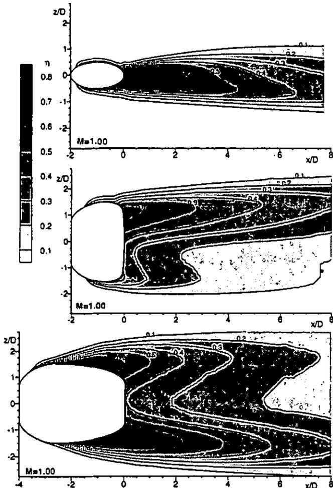
FIG. 12: Local effectiveness  $\eta$  at  $Ma_m=0.6$ ,  $Ma_c=0.6$ ,  $M=1.0$ , and  $\beta=90^\circ$  (a) cylindrical, (b) fanshaped, (c) laidback fanshaped hole (coolant flow approach from down to top)
