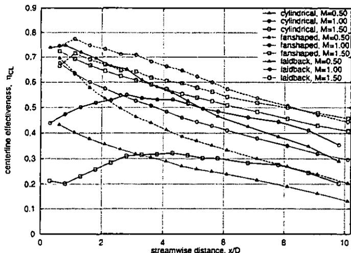
FIG. 5: Centerline effectiveness  $\eta_{CL}$  for the three holes tested at  $Ma_m=0.6$ ,  $Ma_c=0.0$ , and  $\beta=0^\circ$
