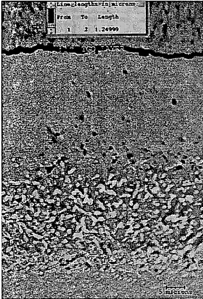
Fig. 2 - Aluminum Oxide Film Grown at EB-PVD TBC Top Coat/Platinum Aluminide Bond Coat Interface for CMSX-4 Specimen
