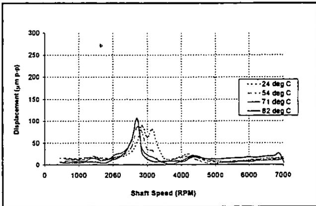
Figure 6. Balanced Condition @ Ry-probe With Metal-Mesh Installed, Multiple Temperatures
