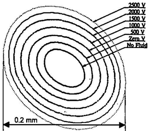
Figure 8: Orbits at the second critical speed with the 350 CS fluid
