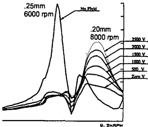
Figure 10: Measured Bode plots with 350 CS fluid (X)
