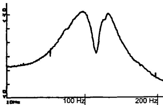
Figure 5: Rap test spectrum, X, 350 CS fluid, no voltage
