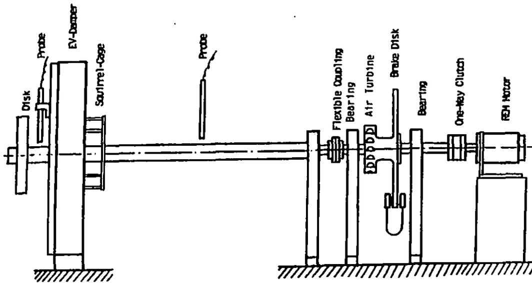
Figure 1: Rotordynamic test rig for the ER damper
