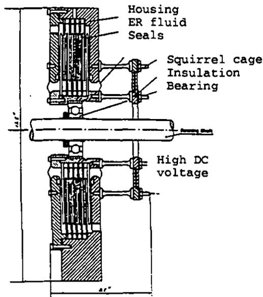
Figure 2: Cross section of the ER damper
