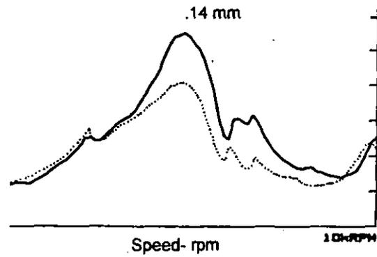
Figure 15: Measured runup response with 10CS fluid and the control system (solid line)
