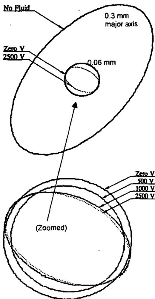
Figure 7: Rotor orbits at the first critical speed with the 350 CS fluid
