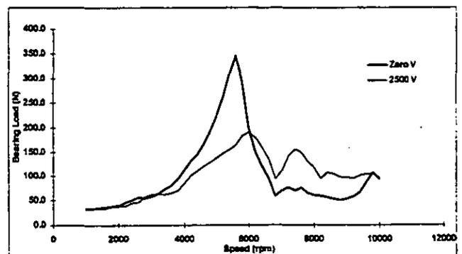
Figure 13: Dynamic bearing loads calculated from the measured stiffness and damping coefficients, 10 CS fluid
