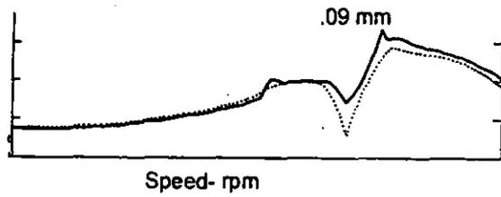
Figure 14: Measured runup response with 350CS fluid and the control system (solid line)
