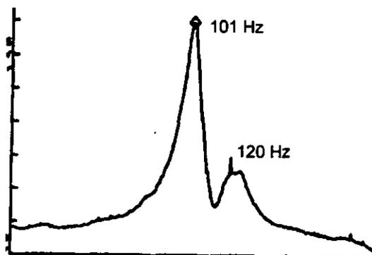
Figure 4: Rap test spectrum, X, no ER fluid
