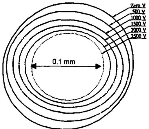
Figure 9: Orbits at the first critical speed with the 10 CS fluid
