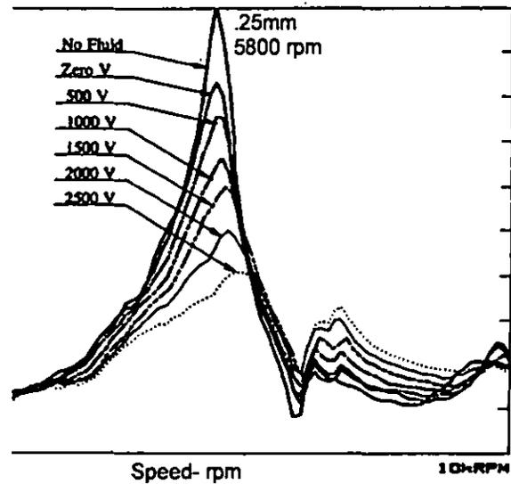
Figure 11: Measured Bode plots with 10 CS fluid (X)
