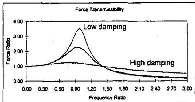
Figure 12: Theoretical dimensionless bearing force vs. frequency ratio for three damping ratios
