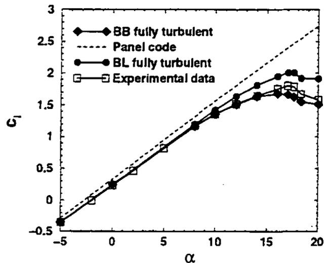
FIG. 2 Lift coefficient versus angle of attack, experimental data by McCroskey et al.
