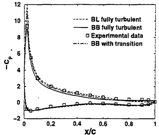
FIG. 6 Pressure coefficient versus chord for  $\alpha = 17.6$  degrees, experimental data by McCroskey et al.
