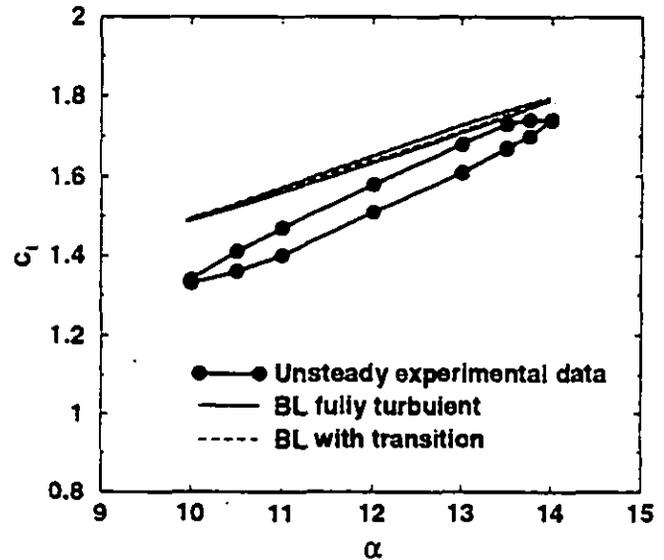
FIG. 12 Unsteady lift coefficient versus angle of attack obtained with the BL model, experimental data by McCroskey et al.
