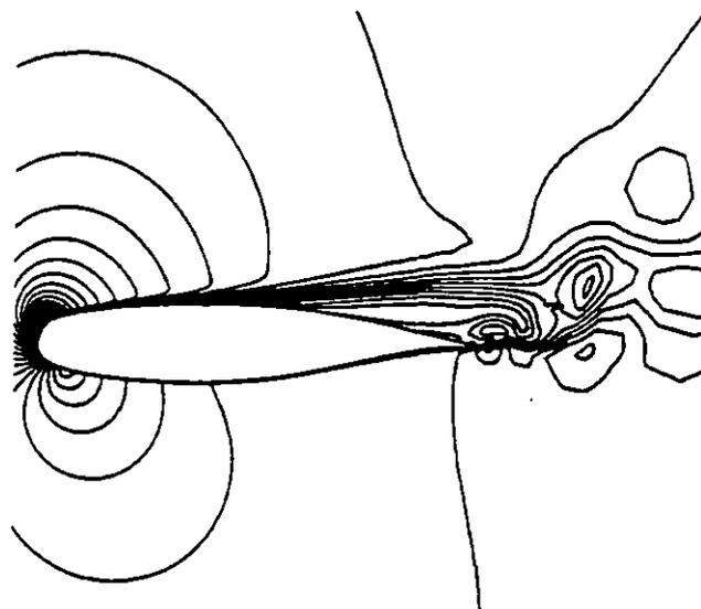
FIG. 9 Instantaneous Mach number distribution for  $\alpha = 20$  degrees computed with the BL model
