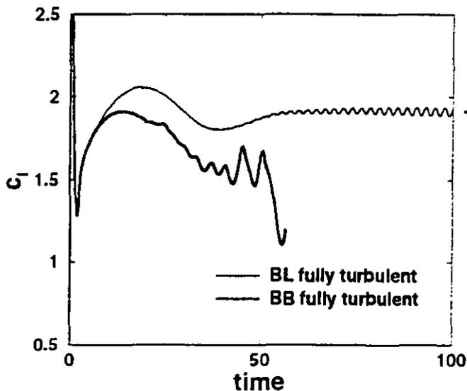
FIG. 8 Time development of the lift coefficient for  $\alpha = 20$  degrees
