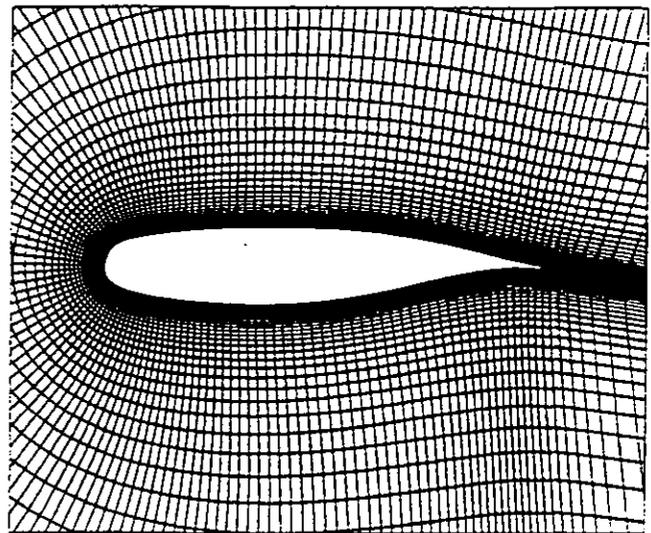
FIG. 1 C-type grid for the NLR 7301 airfoil
