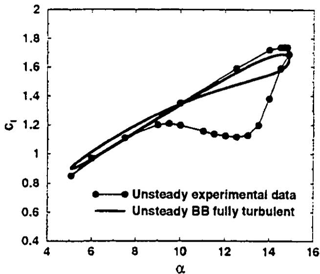
FIG. 18 Fully turbulent unsteady lift coefficient versus angle of attack obtained with the BB model, experimental data by McCroskey et al. for forced turbulent flow
