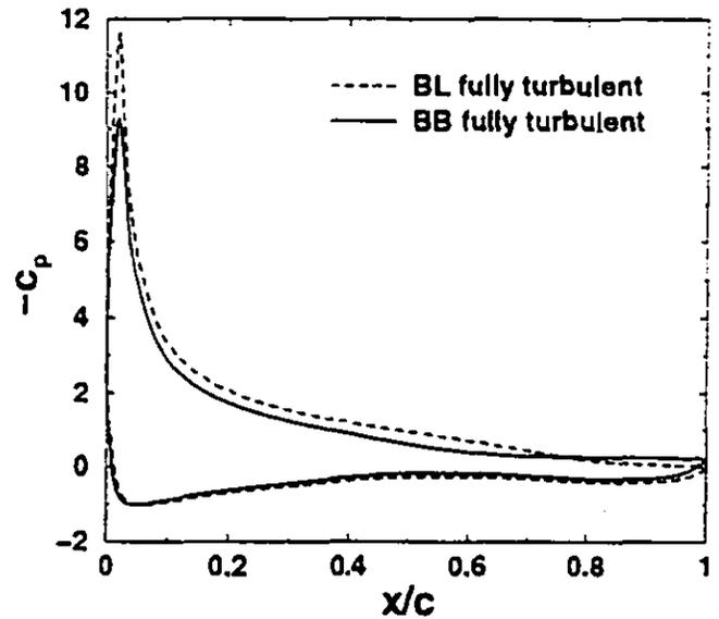
FIG. 5 Pressure coefficient versus chord for  $\alpha = 17$  degrees
