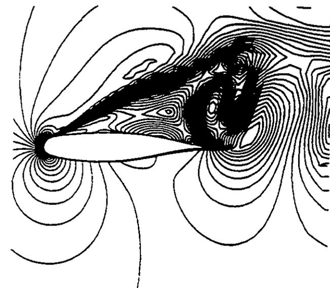
FIG. 10 Instantaneous Mach number distribution for  $\alpha = 20$  degrees computed with the BB model
