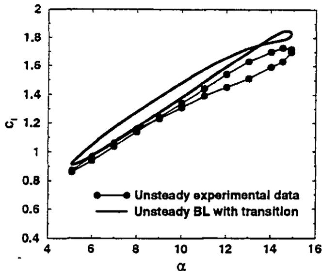
FIG. 15 Unsteady lift coefficient with transition versus angle of attack obtained with the BL model, experimental data by McCroskey et al.
