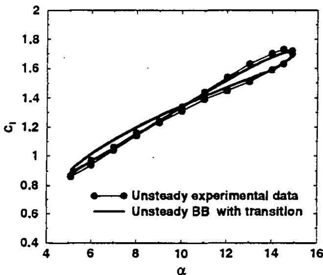
FIG. 16 Unsteady lift coefficient with transition versus angle of attack obtained with the BB model, experimental data by McCroskey et al.
