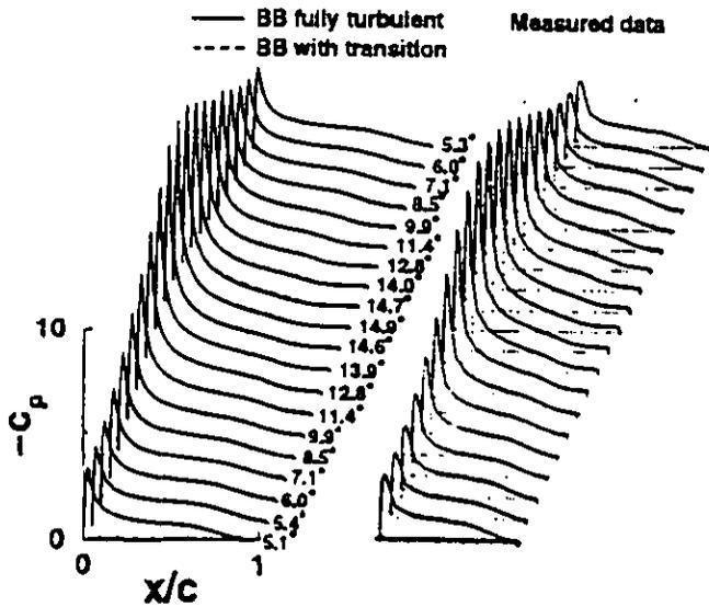
FIG. 17 BB computed unsteady pressure coefficient versus chord in comparison with the measurements by McCroskey et al.
