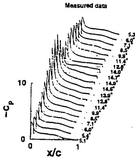
FIG. 19 Unsteady pressure coefficient versus chord for forced fully turbulent flow measured by McCroskey et al.
