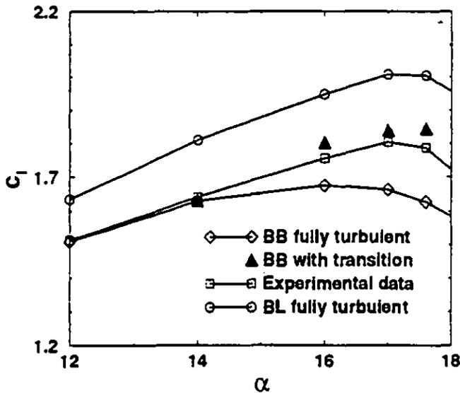
FIG. 11 Lift coefficient versus angle of attack, experimental data by McCroskey et al.
