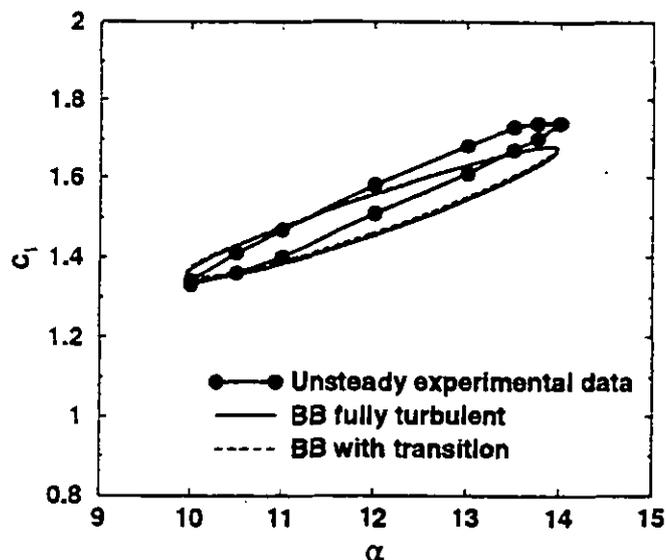
FIG. 13 Unsteady lift coefficient versus angle of attack obtained with the BB model, experimental data by McCroskey et al.
