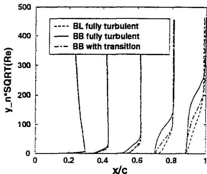
FIG. 7 Boundary layer profiles for  $\alpha = 17.6$  degrees
