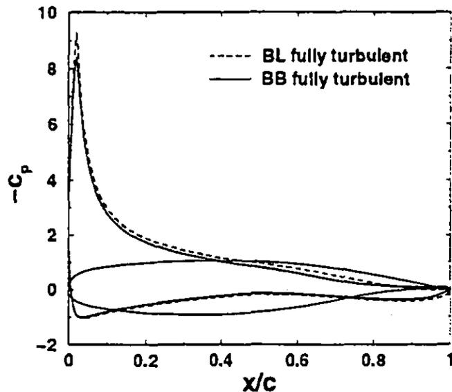
FIG. 4 Pressure coefficient versus chord for  $\alpha = 14$  degrees
