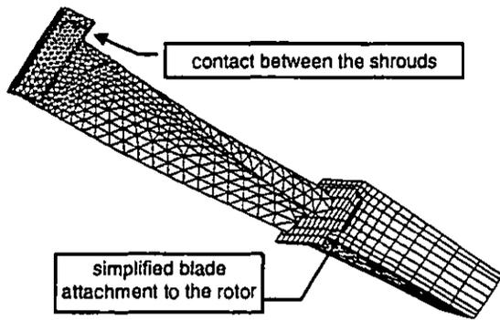
Fig. 5 Cyclic finite element model of the steam turbine blade including the frictional contact between the shrouds
