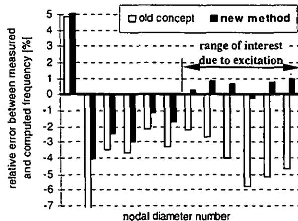
Fig. 8 Relative errors of the computed eigenfrequencies obtained from the traditional (Fig. 1a) and new (Fig. 1c) cyclic finite element models for the turbine blades shown in Fig. 5
