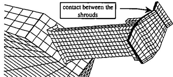
Fig. 3 Cyclic finite element model of the coupled blade including contact between the shrouds
