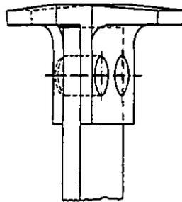
Fig. 2 Analysed disc assembly and details of the shroud assembly at the blade tip (Schaber, 1987)
