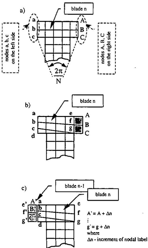
**Fig. 1** Upper part of the two-dimensional mesh of the shrouded blade, a) required symmetrical node configuration for the traditional cyclic finite element model of blade  $n$ , b) asymmetrical node configuration of blade  $n$ , c) proposed cyclic finite element model of the shrouded blade including contact, where  $N$  denotes a blade number in the turbine row
