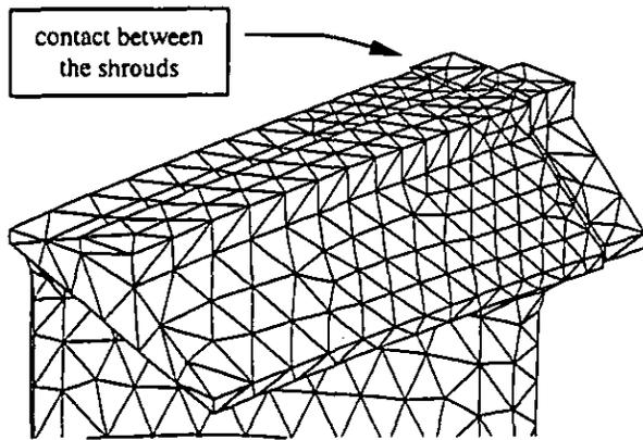
Fig. 6 The deformed configuration between the shrouded blades in the spin pit condition
