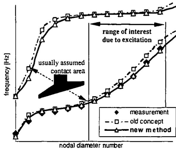
Fig. 7 Calculated and measured (only 1st mode) eigenfrequencies of the shrouded blade in the spin pit measurement
