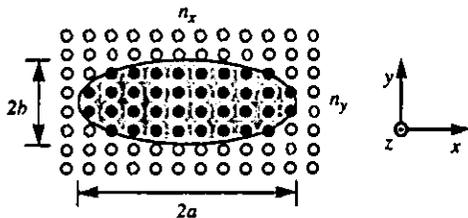
Figure 6 A mesh of  $n_x$  by  $n_y$  bristles, where loaded bristles are shown as filled circles. The area where the indenter is in contact with the foundation is shown in grey.
