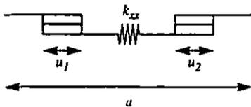
Figure 20 The Bar friction damper model.
