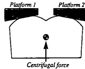
Figure 4 Damper configuration.
