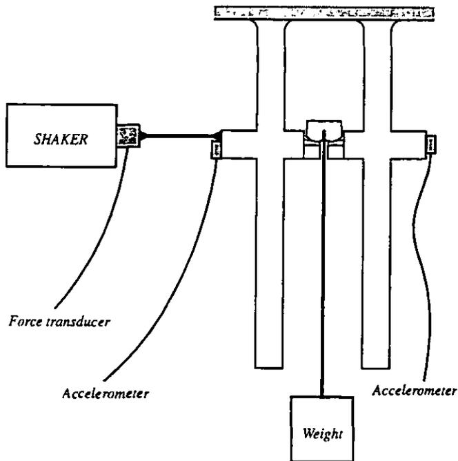
Figure 22 Experimental set-up: Two beams with a damper in between. The left beam is excited by a shaker and response is measured for both beams.
