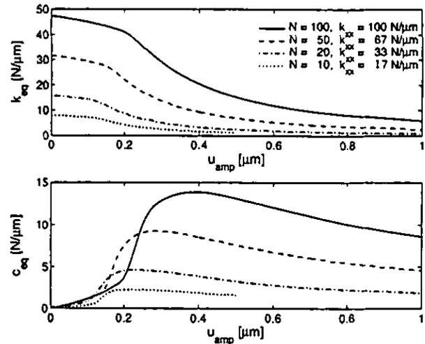
Figure 21 Equivalent stiffness and damping for Brush damper model. Variation of normal force  $N$  and damper stiffness  $k_{xx}$
