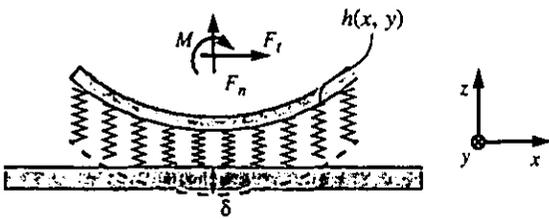
Figure 5 The Brush model, schematic view in two dimensions.
