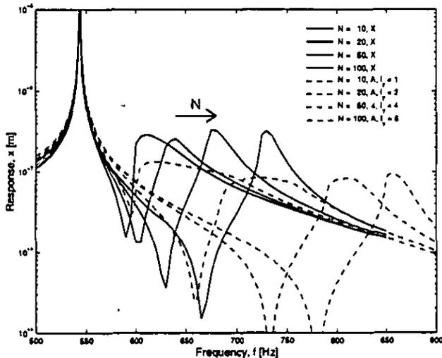
Figure 24 Tracking plots for damper with  $r_x = 2.6$  mm. Experiment (X) vs. analysis (A) varying damper stiffness and contact length.
