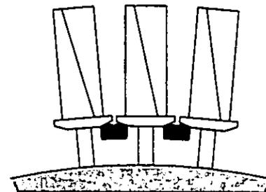
Figure 1 A part of a bladed disk with platform dampers.
