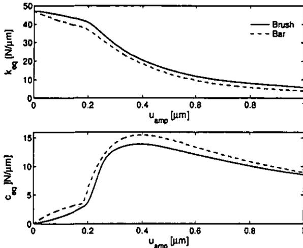
Figure 19 Comparison of equivalent stiffness and damping for Bar and Brush models. Normal force on damper  $N = 100N$ . Radius  $r_x = 2.6$  mm for Brush model.
