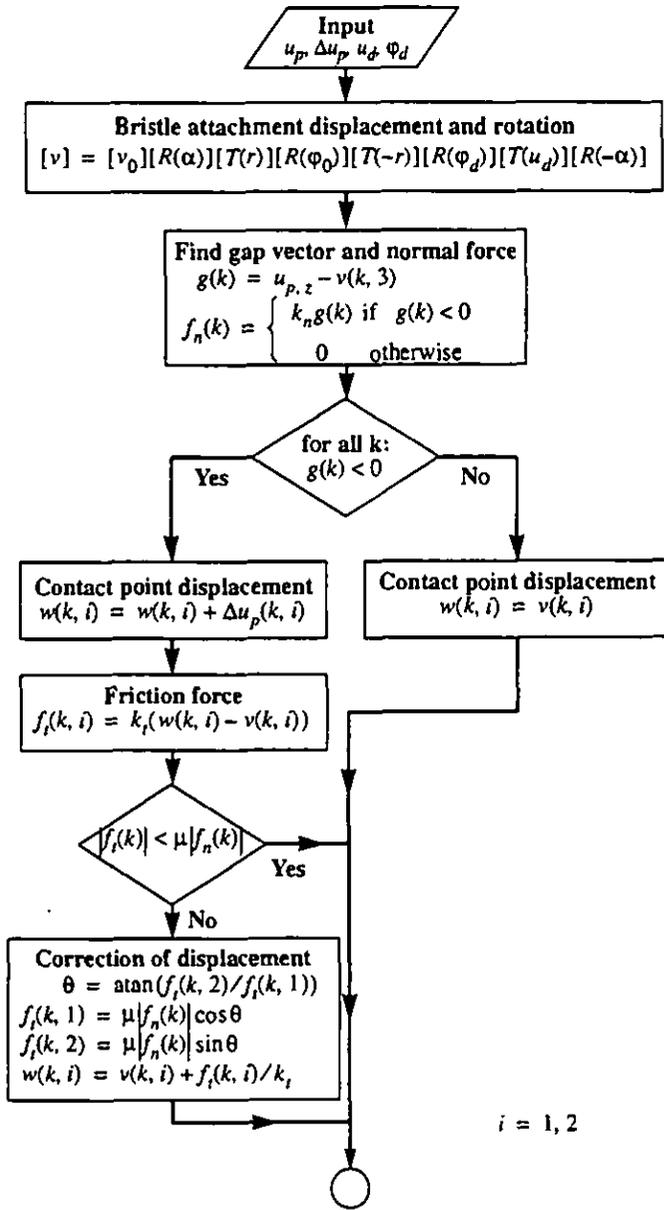
Figure 10 Algorithm for solving bristle force and displacement.
