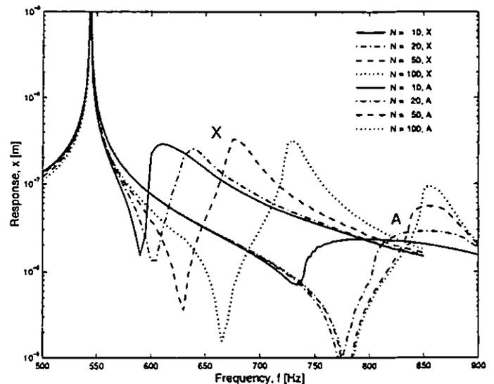
Figure 23 Tracking plots for damper with  $r_x = 2.6\text{ mm}$ , experiment (X) vs. analysis (A)
