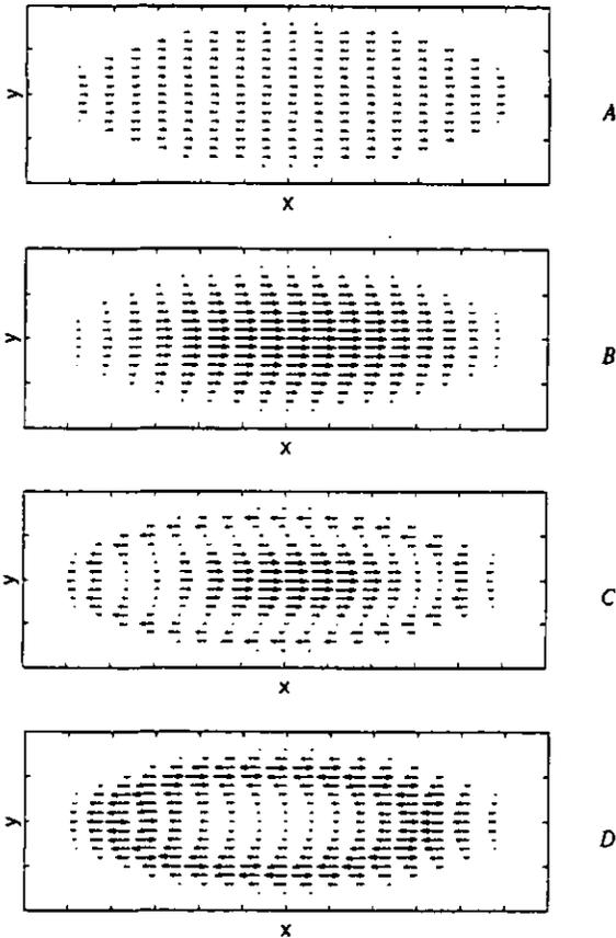
Figure 12 Mesh of bristle friction force for constant normal load simulation.
