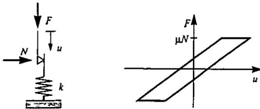
Figure 2 Macroslip friction interface model and corresponding hysteresis curve.
