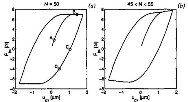
Figure 11 Hysteresis of one friction contact for constant and variable normal load.
