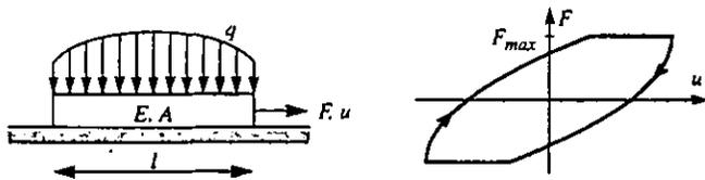
Figure 3 Microslip friction interface model and corresponding hysteresis curve.
