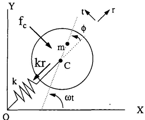
Figure 2: Dynamic force vectors for circular orbits
