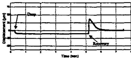
Figure 10 - 25,000 RPM Drop and Recovery on Foil Bearing
