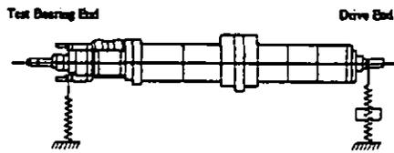
Figure 3 - Rotor Model
