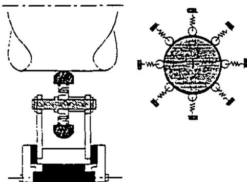
Figure 7 - Zero Clearance Auxiliary Bearing, Concept
