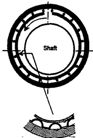
Figure 9 - Foil Bearing Concept
