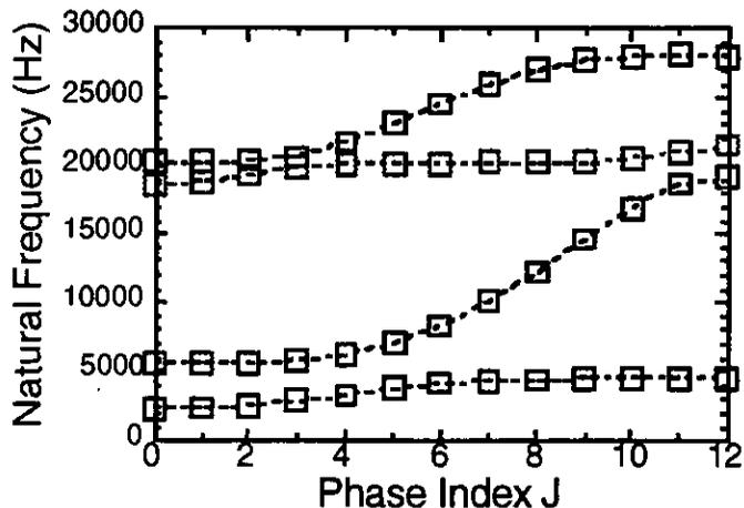
Fig. 3: Natural frequencies of tuned bladed disk
