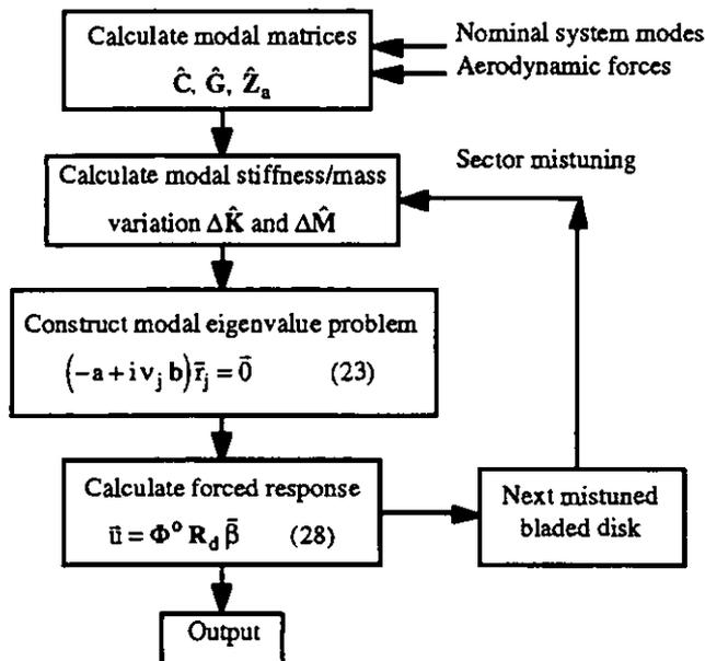
Fig. 1: Flow chart for the SNM algorithm
