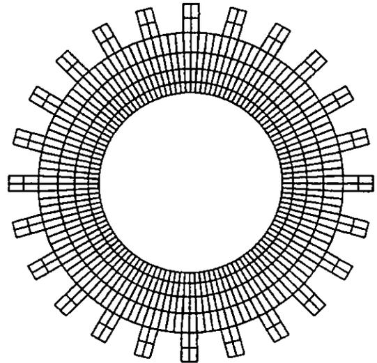
Fig. 2: Finite element model of bladed disk system
