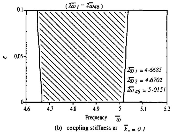
Figure 6 The variations in the transition curves for different rotating speeds
