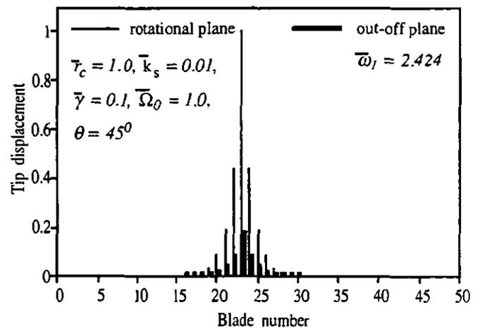
Figure 2 Tip displacement patterns of a cracked blade-disk system
