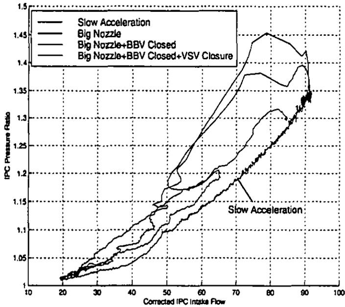
Fig. 1: Means for Validation of Surge Margin
