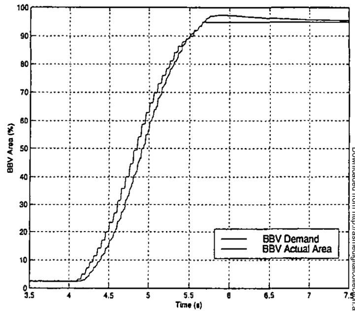
Fig. 4: BBV Opening Rate Limiter impact
