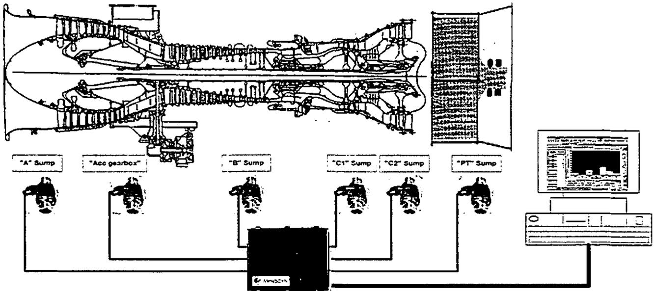
Figure 3 - Chalk Cliff MetalSCAN Installation
