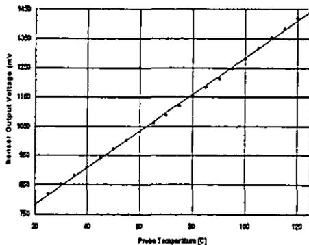
Figure 5 Multilayer sensor calibration, 20 to  $120\text{ }^\circ\text{C}$ , using a laser diode wavelength of  $792\text{ nm}$
