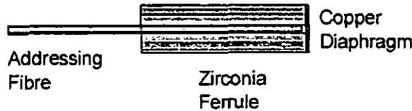
Figure 7 Pressure sensor schematic.
