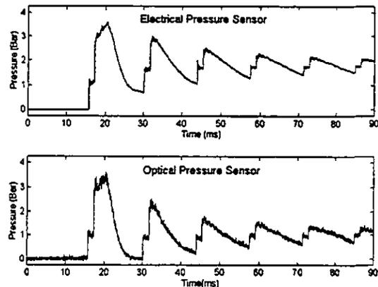
**Figure 11 Shock tube pressure-time signals (upper) electrical sensor; (lower) optical sensor**
