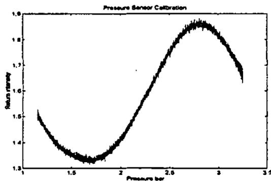
Figure 8 Reflected optical signal as a function of pressure
