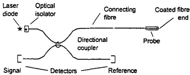
Figure 4 Optical system of the temperature sensor
