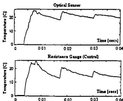
**Figure 10 Shock tube test of (upper) optical temperature sensor compared with (lower) Pt thin film gauge in forward-facing total temperature probe**
