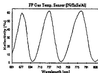
Figure 3 Wavelength scan of (Ni-ZnSe-Al) multilayer
