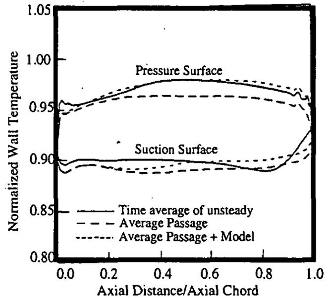
Fig. 8. Turbine blade temperature distribution.
