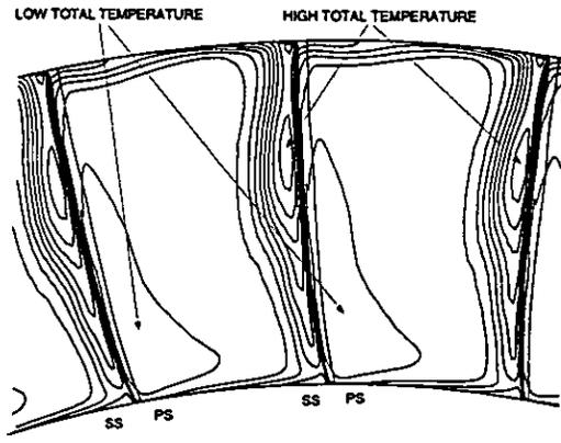
Fig. 4a. Total temperature exiting a high speed compressor rotor at an instant of time.
