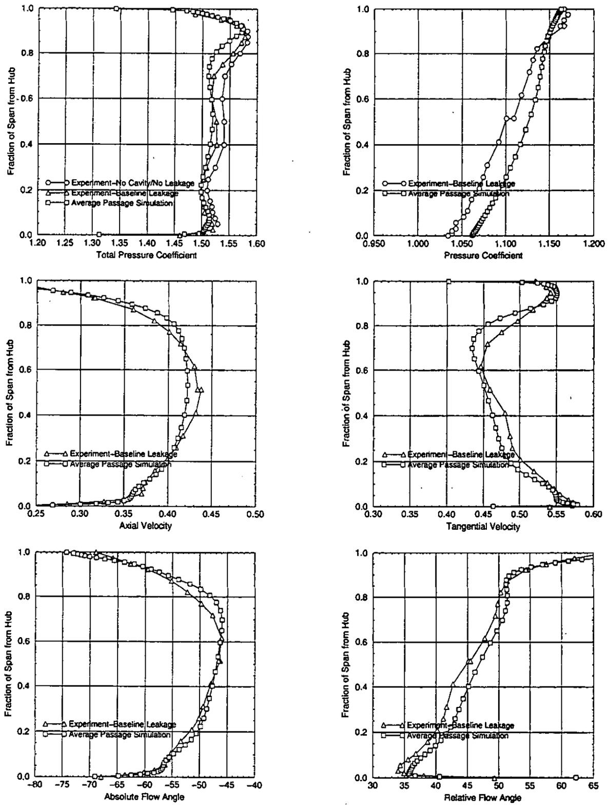
Fig. 13. Axisymmetric flow variables exiting the 3rd stage rotor in the NASA-Lewis low speed four-stage axial compressor.
