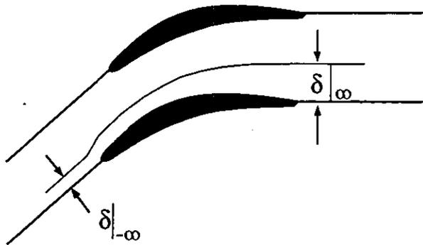
Fig. 27. Steady flow through a cascade with blockage.
