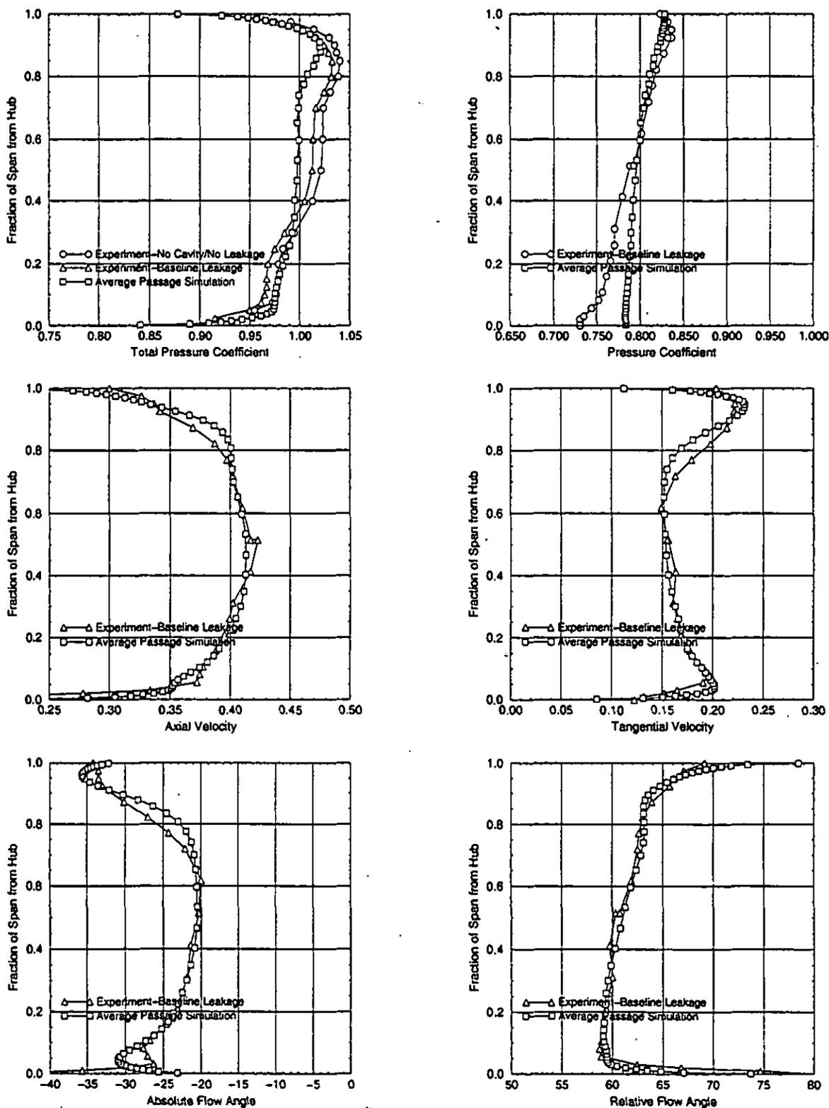
Fig. 12. Axisymmetric flow variables exiting the 2nd stage stator in the NASA-Lewis low speed four-stage axial compressor.
