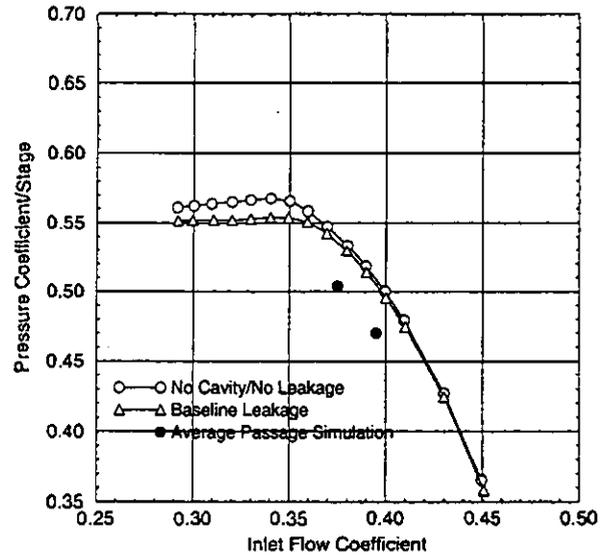
Fig. 28. Overall pressure coefficient as a function of inlet flow coefficient for the NASA-Lewis four stage axial flow compressor.
