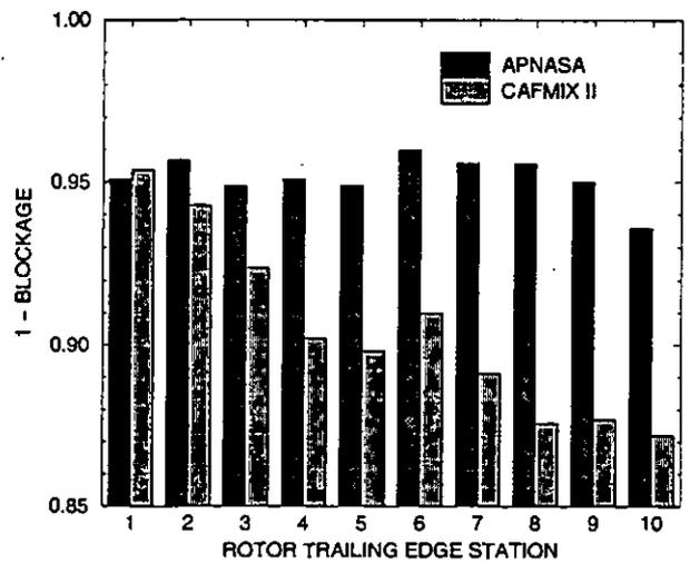
Fig. 16. Flow blockage distribution through the GE90 compressor.
