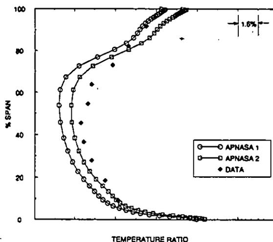
Fig. 24b. Spanwise distribution of total temperature at the exit of the stage 3 rotor for a 3-stage high speed compressor.
