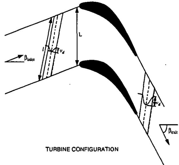
Fig. 9. Wake blade row interactions in a typical turbine and compressor.
