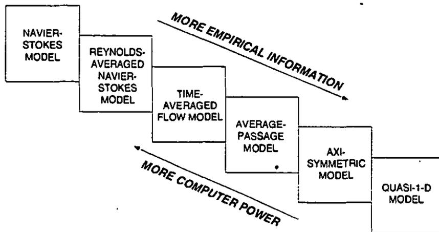
Fig. 1. The range of mathematical models which can be used to simulate turbomachinery flows.
