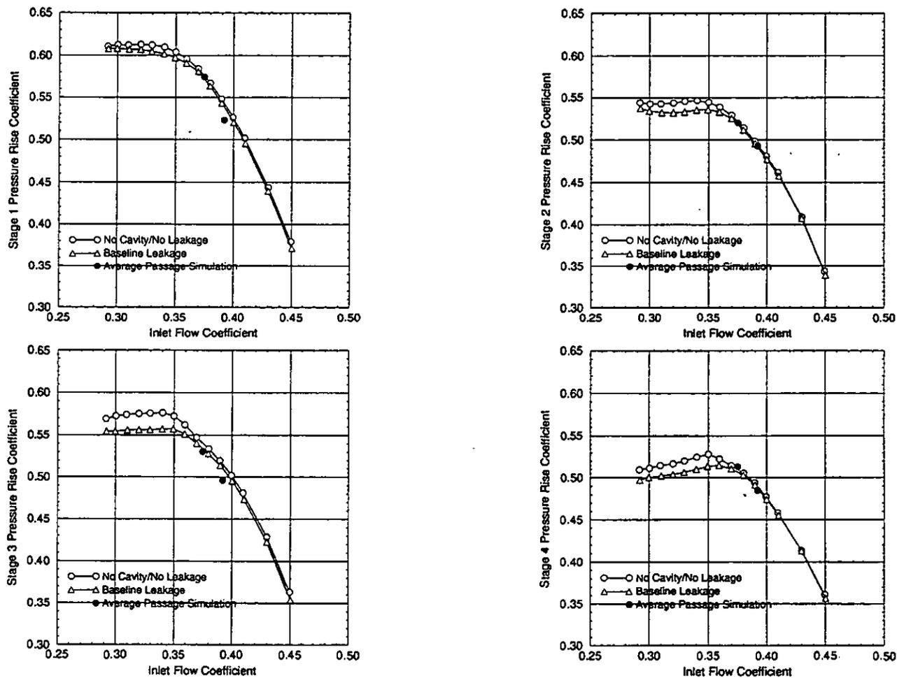
Fig. 11. Individual stage pressure rise coefficient as a function of inlet flow coefficient for the NASA-Lewis low speed four-stage axial compressor.
