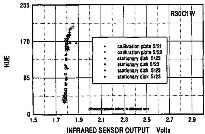
FIG 3 VARIATION OF HUE FOR NARROW-BAND TLC WITH VOLTAGE OUTPUT OF INFRA-RED SENSOR (STATIONARY MEASUREMENT)
