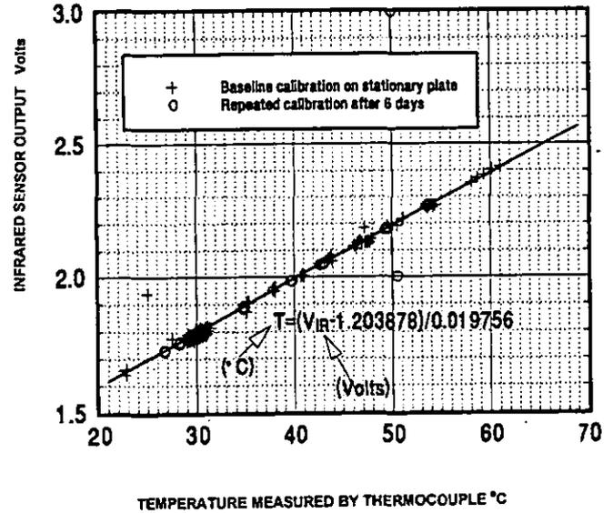
FIG 2 VARIATION OF VOLTAGE OUTPUT OF INFRA-RED SENSOR WITH TEMPERATURE MEASURED BY THERMOCOUPLE IN STATIONARY PLATE
