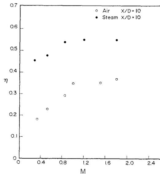
Fig. 10 Steam and Air Cooling Effectiveness Versus Blowing Rate for Position X/D=10
