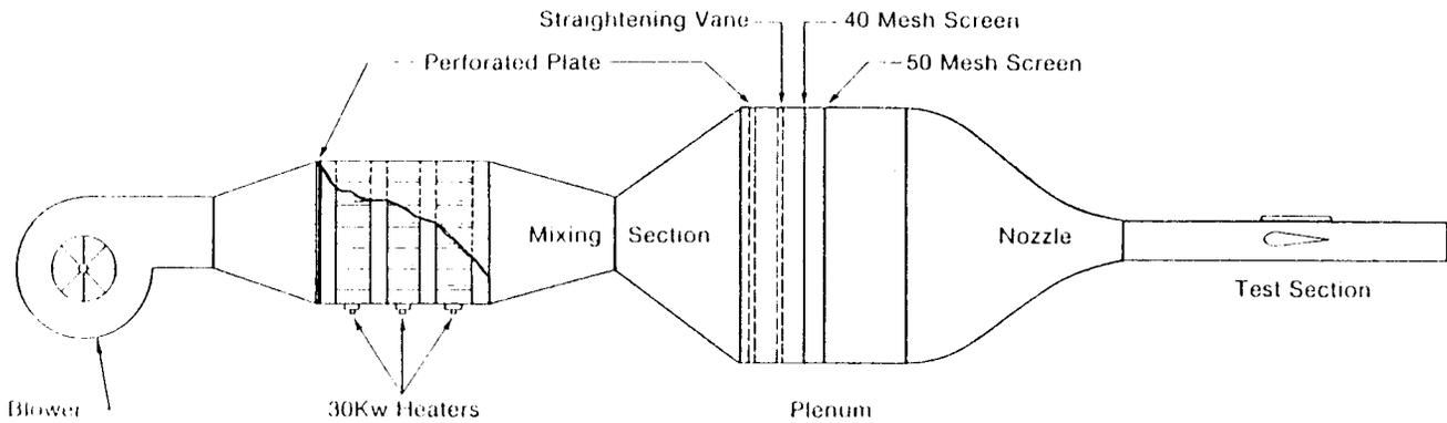
Figure 1 Schematic of the Test Apparatus
