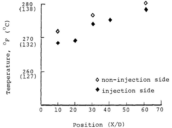
Figure 6 Thermocouple Correlation for an Uncooled Blade
