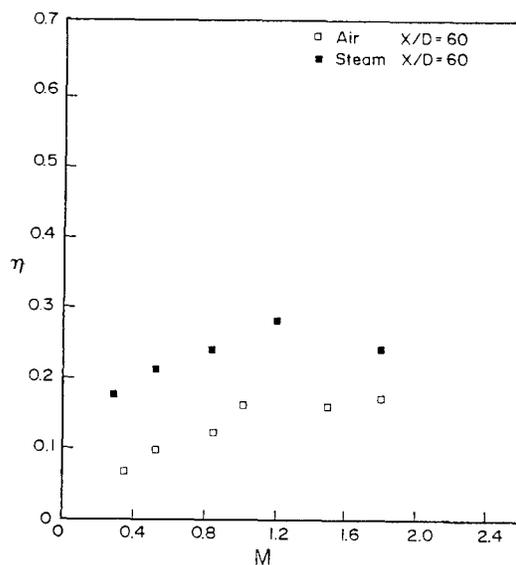
Fig. 12 Steam and Air Cooling Effectiveness Versus Blowing Rate for Position X/D=60
