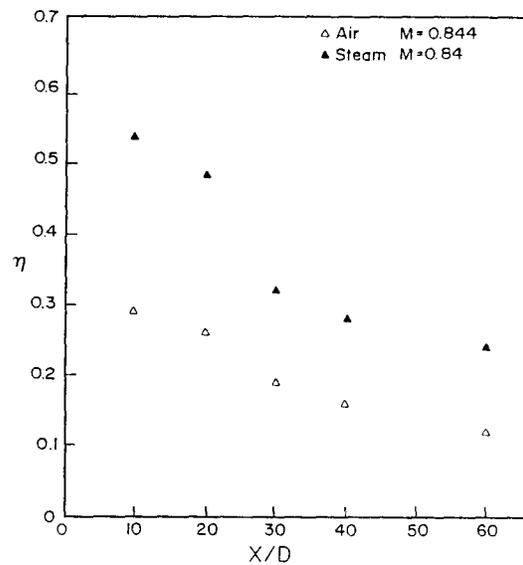
Fig. 8 Steam and Air Effectiveness for Blowing Rates at Different Positions
