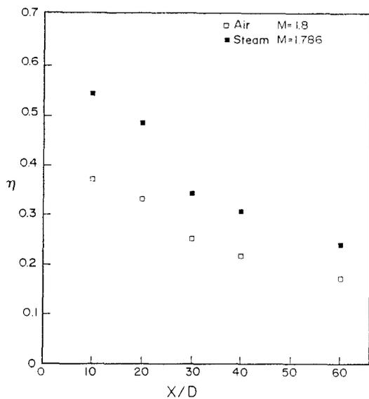
Fig. 9 Steam and Air Effectiveness for Blowing Rates at Different Positions
