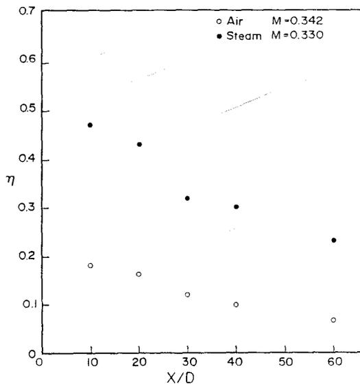
Fig. 7 Steam and Air Effectiveness for Blowing Rates at Different Positions
