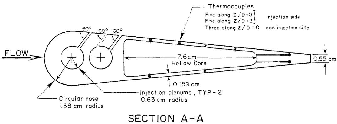
Fig. 4 Sketch of present Injection Geometry
