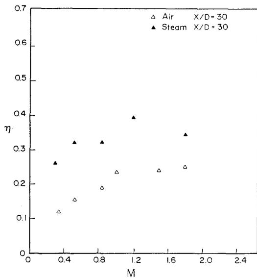
Fig. 11 Steam and Air Cooling Effectiveness Versus Blowing Rate for Position X/D=30
