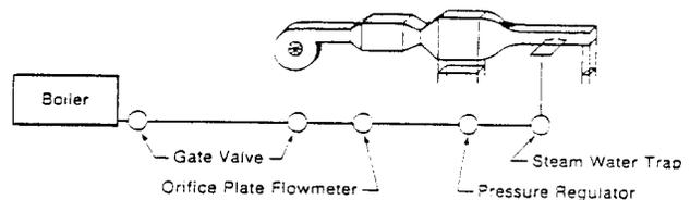
Figure 5 Piping Network Schematic
